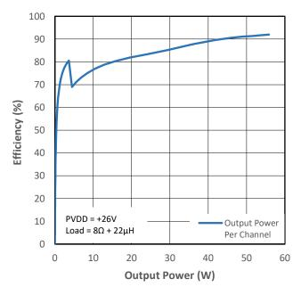
Figure 11-11 PMP2 Efficiency (VDD+PVDD) vs Output Power
