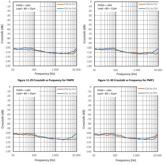
Figure 11-31 Crosstalk vs Frequency for PMP2
