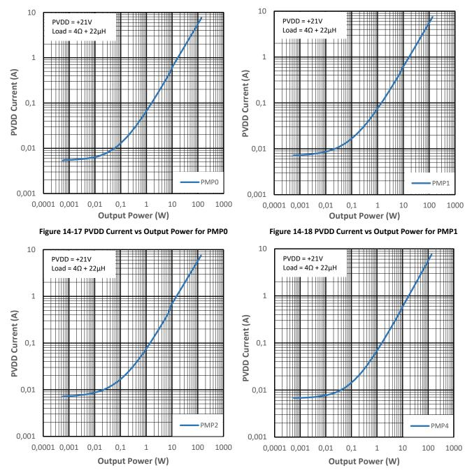
Figure 14-19 PVDD Current vs Output Power for PMP2
