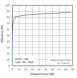
Figure 10-12 PMP4 Efficiency (VDD+PVDD) vs Output Power
