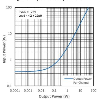
Figure 10-16 Input Power vs Output Power for PMP4
