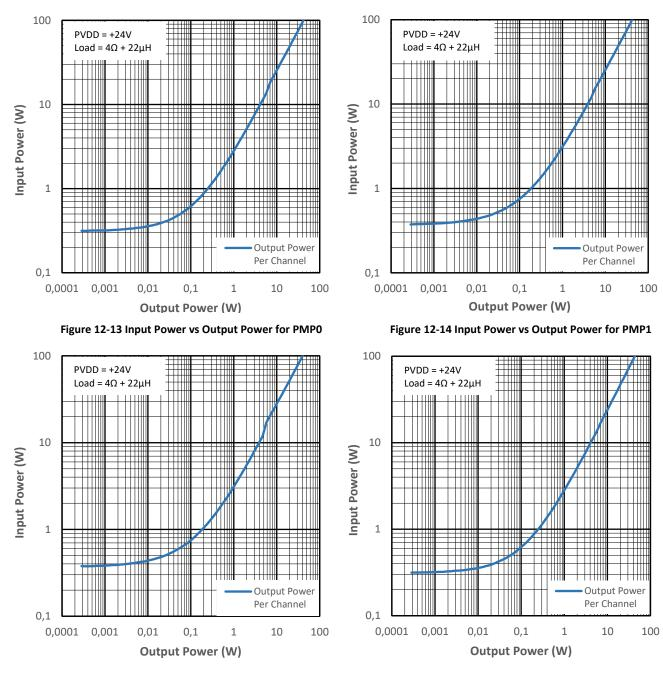
Figure 12-15 Input Power vs Output Power for PMP2
