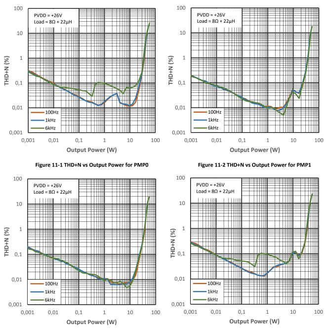
Figure 11-3 THD+N vs Output Power for PMP2
