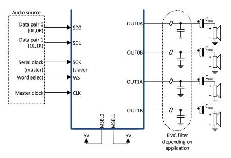
Figure 9-2 Four channel, single ended (SE) configuration.
