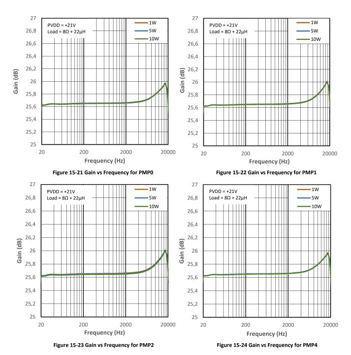
**BTL configuration;** Load =  $8\Omega$  +  $22\mu$ H; Measurements carried out with APx 515 + AUX-0025 input filter; APx uses AES17 brick-wall filter (20kHz).
