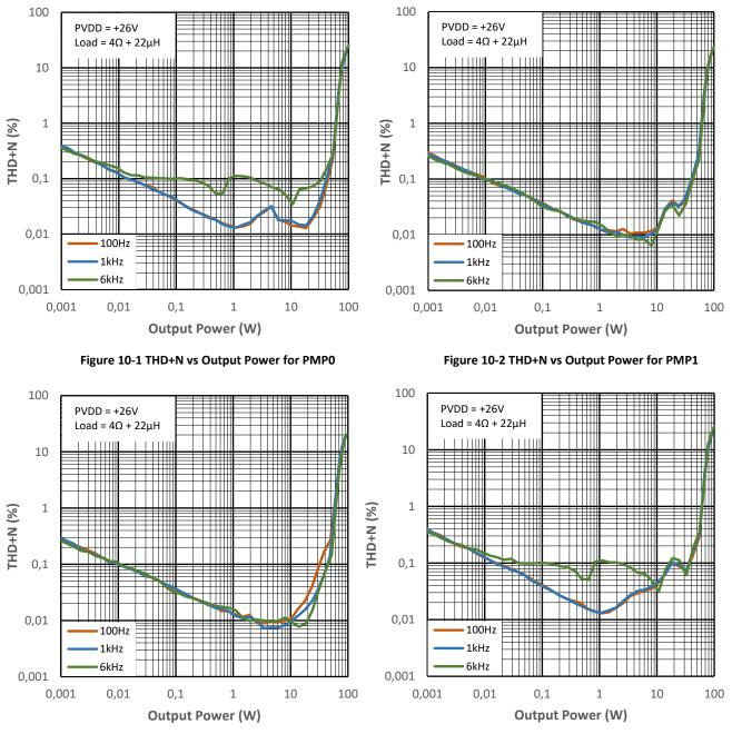
Figure 10-3 THD+N vs Output Power for PMP2
