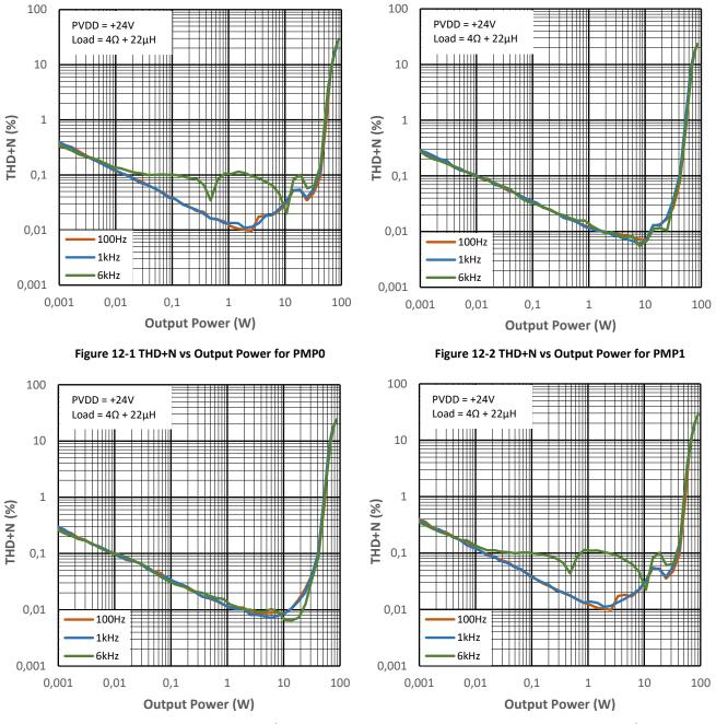
Figure 12-3 THD+N vs Output Power for PMP2
