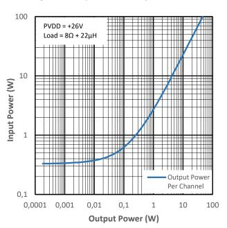
Figure 11-16 Input Power vs Output Power for PMP4
