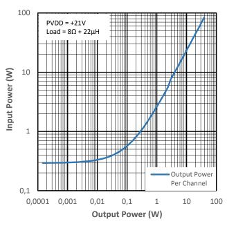
Figure 15-13 Input Power vs Output Power for PMP0
