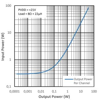
Figure 15-16 Input Power vs Output Power for PMP4
