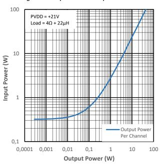
Figure 14-16 Input Power vs Output Power for PMP4
