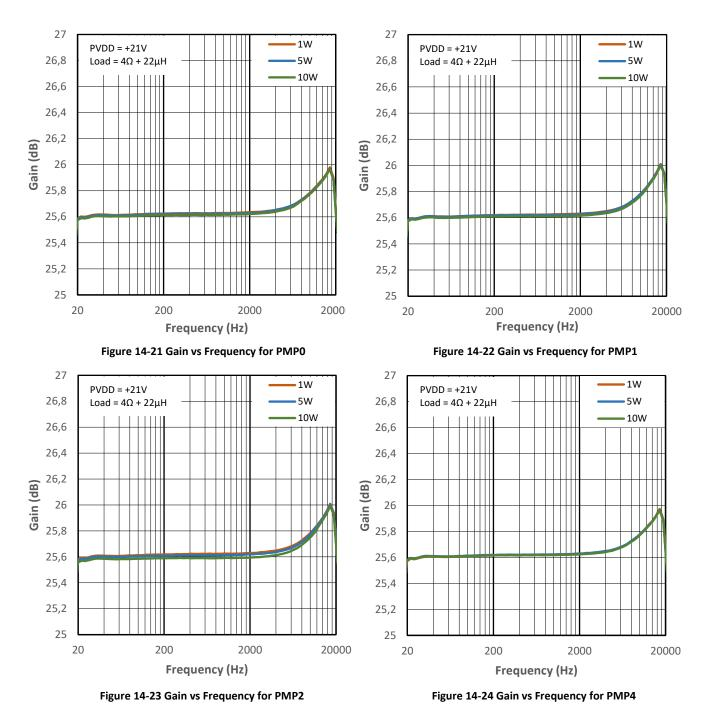
**BTL configuration;** Load =  $4\Omega + 22\mu$ H; Measurements carried out with APx 515 + AUX-0025 input filter; APx uses AES17 brick-wall filter (20kHz).
