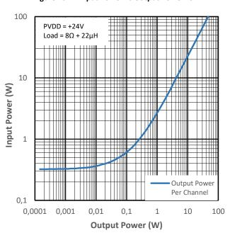
Figure 13-16 Input Power vs Output Power for PMP4
