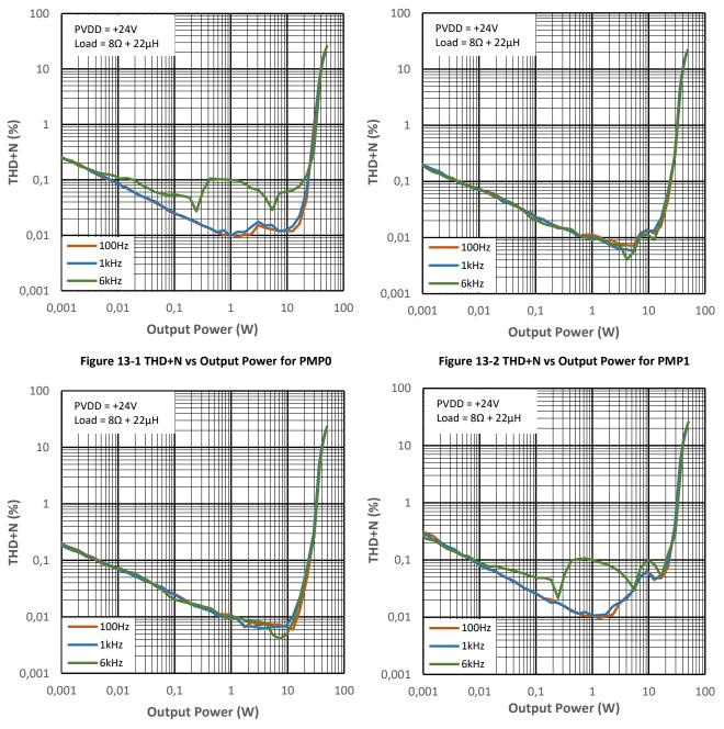
Figure 13-3 THD+N vs Output Power for PMP2
