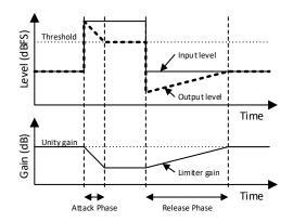
Figure 8-6 Example of limiter attack - and release behavior
