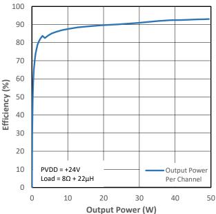
Figure 13-12 PMP4 Efficiency (VDD+PVDD) vs Output Power
