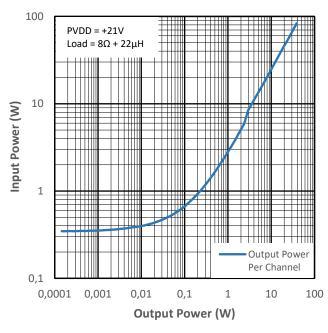
Figure 15-15 Input Power vs Output Power for PMP2
