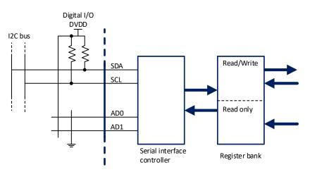
Figure 8-7. I2C bus interface and register bank
