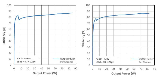
**BTL configuration;** Load =  $4\Omega + 22\mu$ H; Measurements carried out with APx 515 + AUX-0025 input filter; APx uses AES17 brick-wall filter (20kHz).
