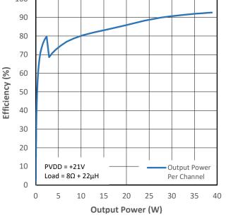
Figure 15-11 PMP2 Efficiency (VDD+PVDD) vs Output Power
