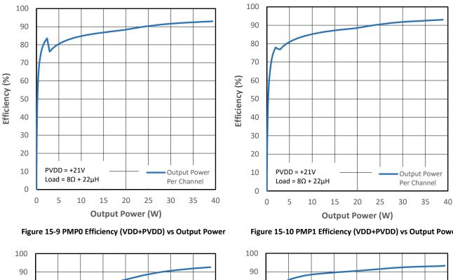
BTL configuration; Load =  $8\Omega$  +  $22\mu$ H; Measurements carried out with APx 515 + AUX-0025 input filter; APx uses AES17 brick-wall filter (20kHz).
