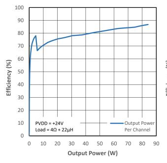
Figure 12-11 PMP2 Efficiency (VDD+PVDD) vs Output Power
