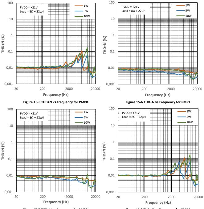
Figure 15-7 THD+N vs Frequency for PMP2
