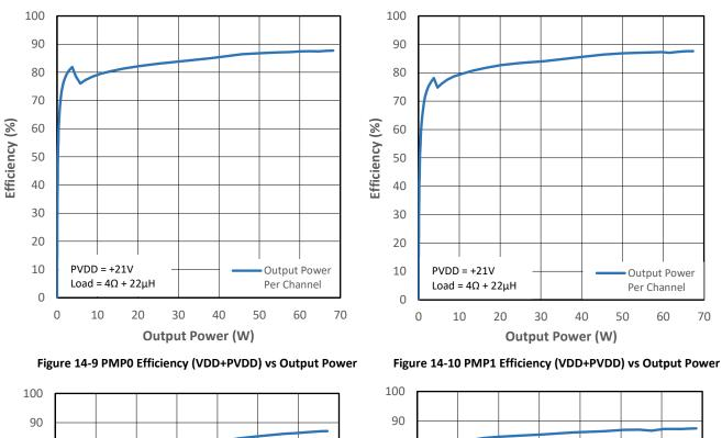
BTL configuration; Load =  $4\Omega$  +  $22\mu$ H; Measurements carried out with APx 515 + AUX-0025 input filter; APx uses AES17 brick-wall filter (20kHz).
