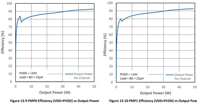
BTL configuration; Load =  $8\Omega$  +  $22\mu$ H; Measurements carried out with APx 515 + AUX-0025 input filter; APx uses AES17 brick-wall filter (20kHz).
