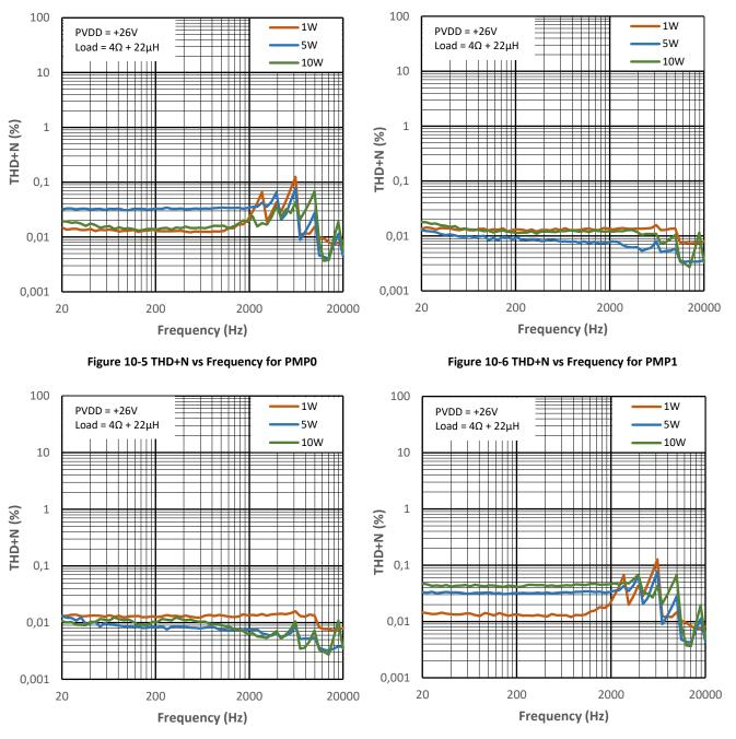
Figure 10-7 THD+N vs Frequency for PMP2
