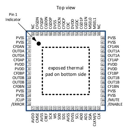
Figure 4-1 Pinout MA12070P
