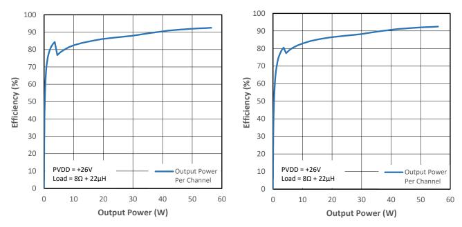
**BTL configuration;** Load =  $8\Omega$  +  $22\mu$ H; Measurements carried out with APx 515 + AUX-0025 input filter; APx uses AES17 brick-wall filter (20kHz).
