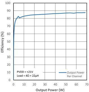
Figure 14-12 PMP4 Efficiency (VDD+PVDD) vs Output Power
