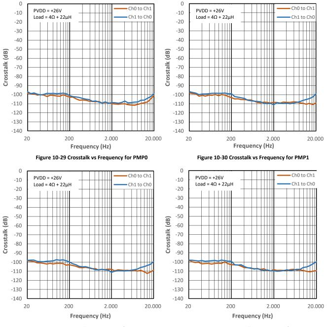
Figure 10-31 Crosstalk vs Frequency for PMP2
