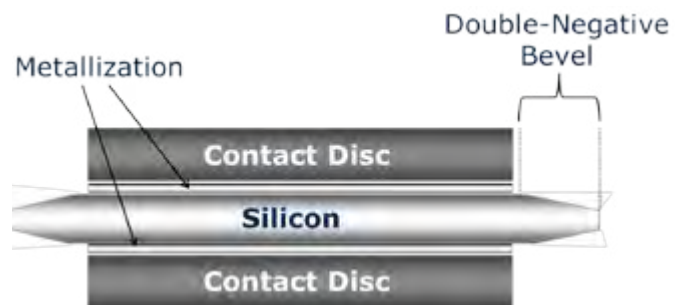
Figure 2b: Cross-section of FF design and double-side negative bevel
