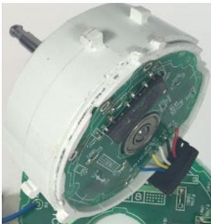
Figure 1: Example of a restricted environment where the PCB is mounted inside the motor
