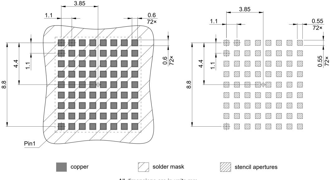
All dimensions are in units mm Based on stencil thickness 0.13 mm All pads are solder mask defined
