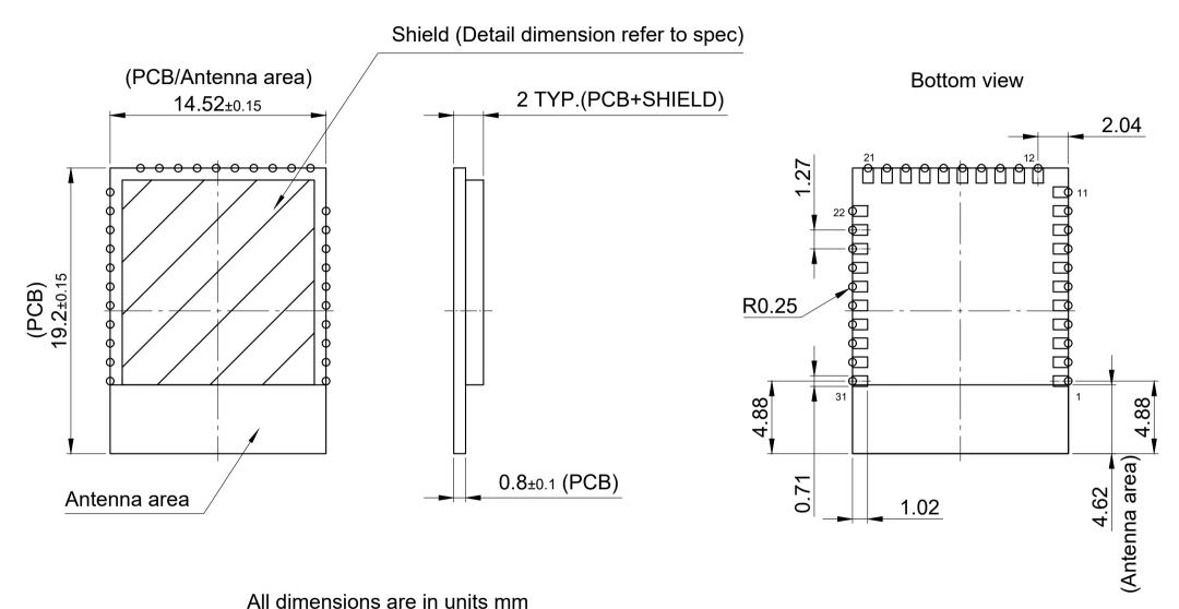
The drawing is in compliance with ISO 128-30, Projection Method 1 [ $\bigcirc \oplus$ ]
