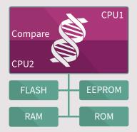
The dual-CPU processor core allows comprehensive error detection
