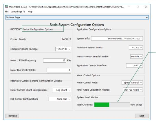
For customized design, total CPU load will change according to PWM frequency and other configuration options.
