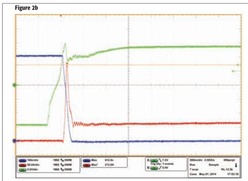
**Figure 2: Commutation of low currents at 10 % of nominal current level (a:  $R_{Gon} = 0\Omega$ , b:  $R_{Gon} = 1.5\Omega$ ;  $V_{CE} = 600V$ ;  $I_c = 60A$ ;  $-15V < V_{GE} < 15V$ ) with collector-emitter voltage (blue), collector current (red) and gate-emitter voltage (green) with a standard gate driver**
