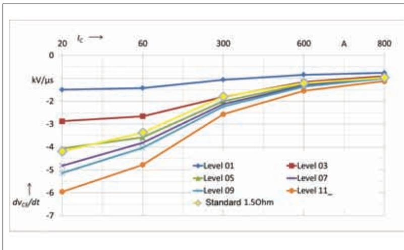
Figure 5: Example of  $dv_{CE}/dt$  range (bottom) and turn-on energy  $E_{on}$  of 1EDS-SRC gate current control IC for speed level 1, 3, 5, 7, 9 and 11 compare to standard driver at IGBT junction temperature of 25°C
