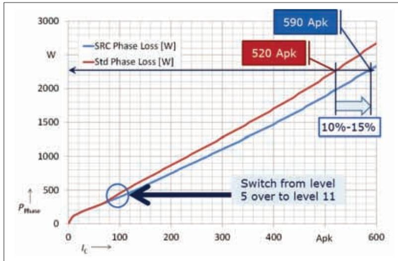
**Figure 6:** Calculated power losses per phase show a gain of 10 % - 15 % in respect to output current with slew rate control (blue) over a standard driver (red) ( $V_{DC} = 600 \text{ V}$ ,  $-8 \text{ V} < V_{GE} < 15 \text{ V}$ ,  $f_r = 15 \text{ kHz}$ )
