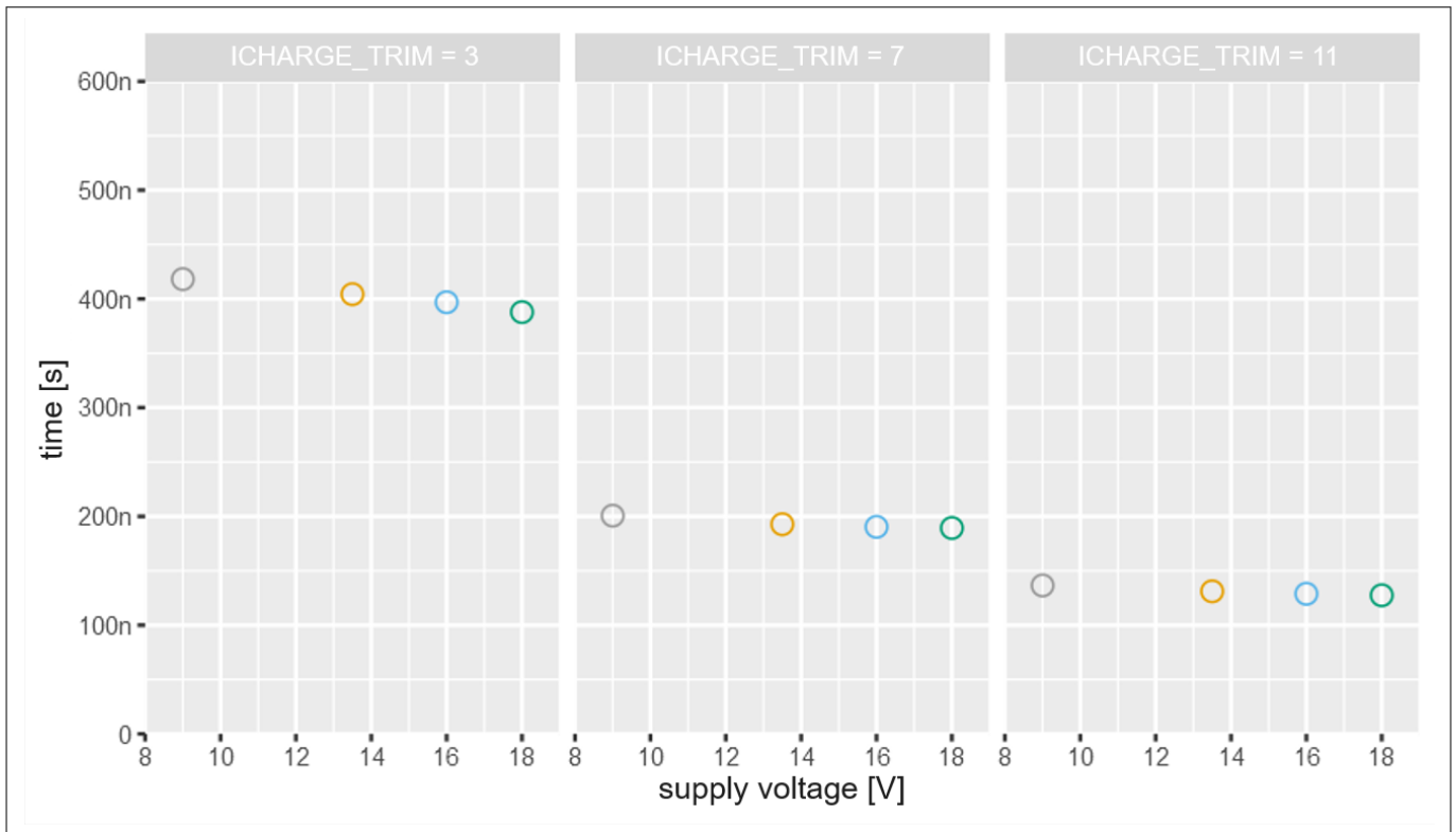
Figure 66 The plot shows the turn ON delay for low-side MOSFETs when it is tested with a gate driver at 25°C temperature and 30 A load current
