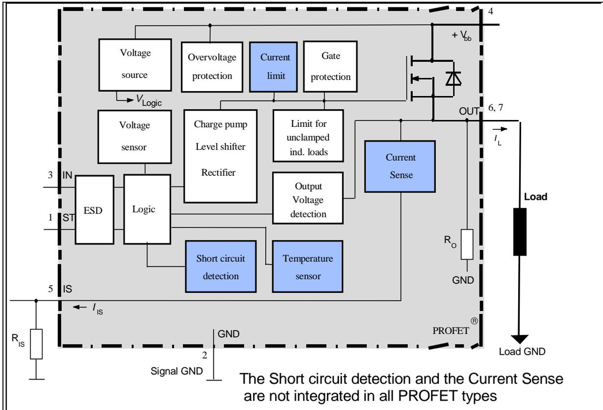
**Figure 3** Block diagram of PROFET highside switches
