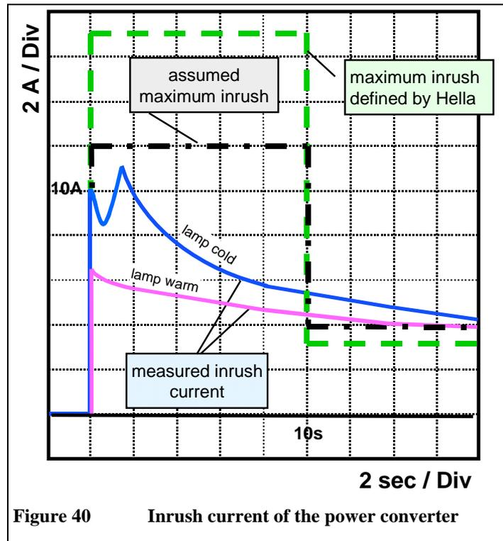
Figure 40 Inrush current of the power converter
