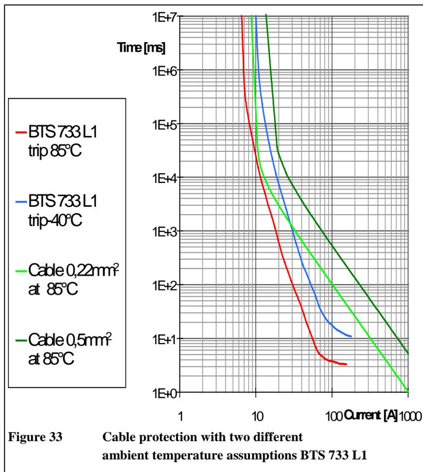
temperature dependence. Fig. 33 shows the trip characteristics of a BTS 733 L1 (at -40°C and at 85°C) and two cables with different diameters at 85°C. This illustrates the large extent to which the "inverse ambient temperature assumption" influences the dimensioning of the PROFET or cable. It is advisable to consider whether this extreme case can occur at all and whether this assumption is necessary.
