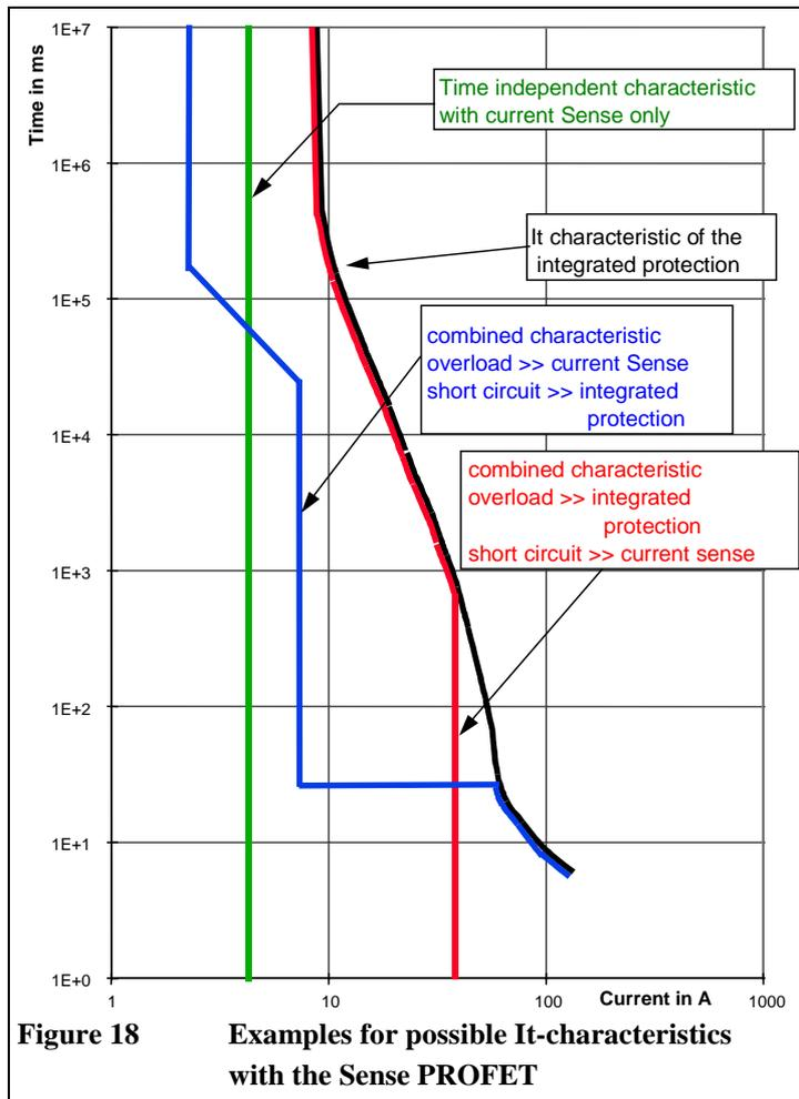
**Figure 18** Examples for possible  $I_t$ -characteristics with the Sense PROFET
