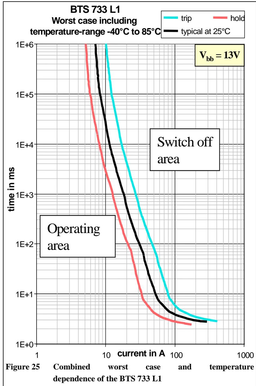
Figure 25 Combined worst case and temperature dependence of the BTS 733 L1
