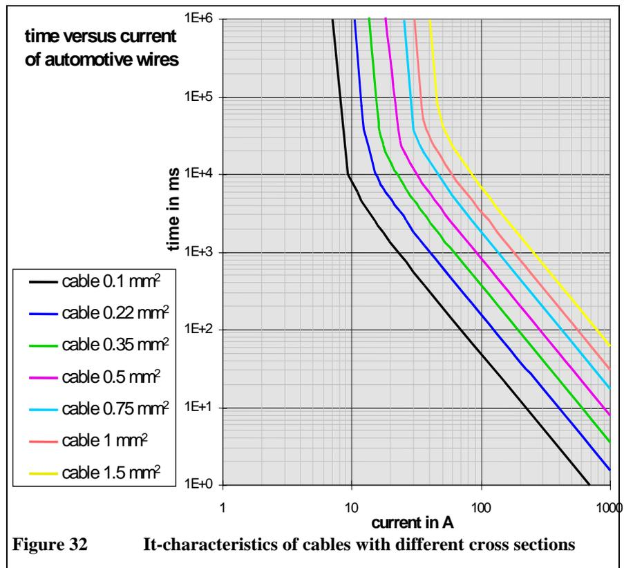
**Figure 32** It-characteristics of cables with different cross sections
