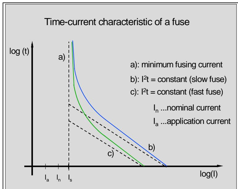
**Figure 1** Approximation of It-characteristic by two asymptotic lines
