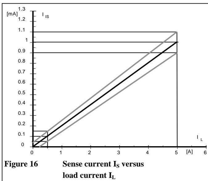
Figure 16 Sense current  $I_S$  versus load current  $I_L$
