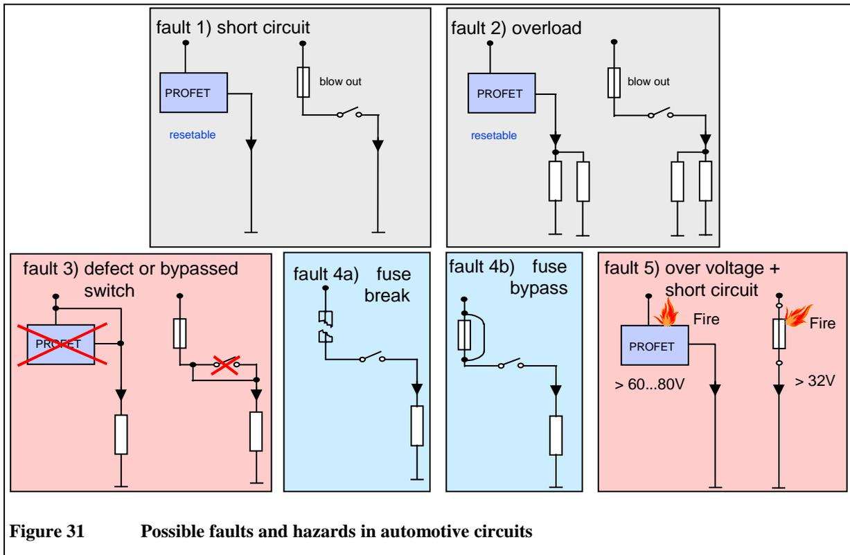
Figure 31 Possible faults and hazards in automotive circuits
