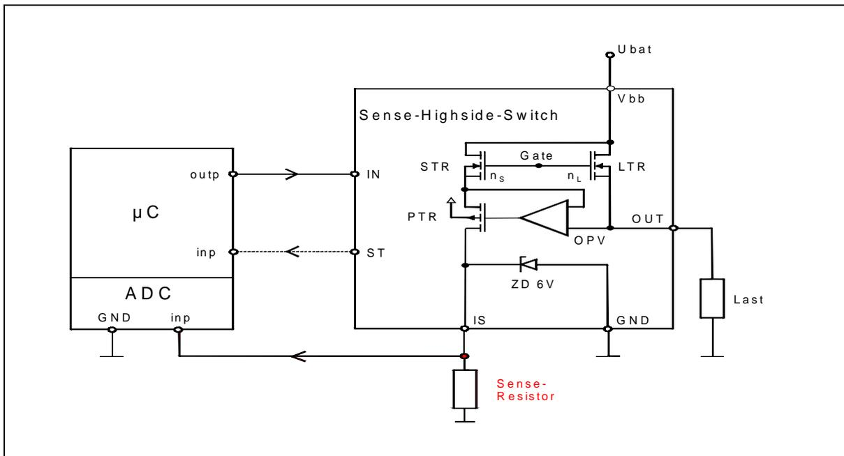
Figure 15 Circuit diagram of the Sense principle (BTS 640 S2)
