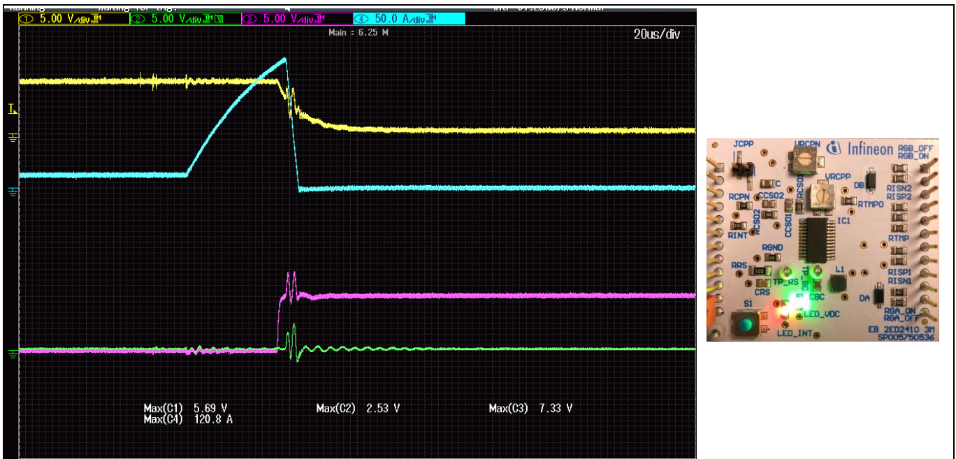
Figure 19 Waveforms from ON to SAFESTATE [Yellow V_{IN} ; Green V_{DG0} ; Purple V_{DG1} ; Blue V_{GS} ]
