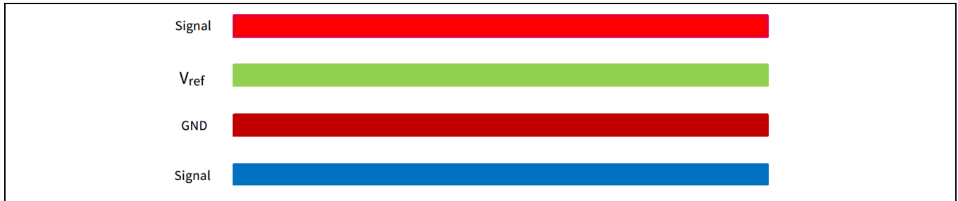
Figure 30 EB 2ED2410 3M PCB layers 4 * 35µm
