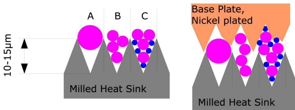
Figure 3: Influence of material properties to the forming of contact areas
