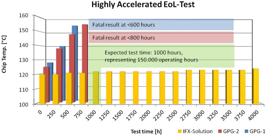
Figure 5: Results from the accelerated stress test, simulating 20 years of operation
