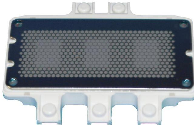
Figure 4: EconoPACK™ 4 with TIM applied. Stencil printing enables the application of locally optimized volumes using inhomogeneous patterns.
