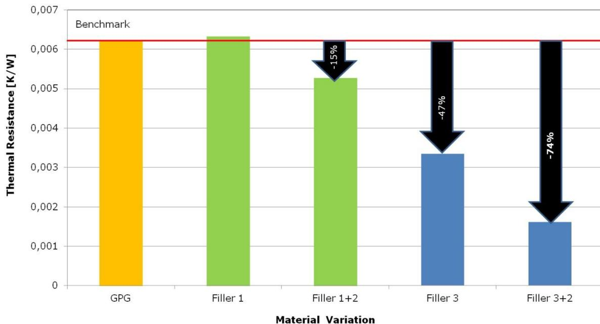
Figure 2: Comparing thermal resistances of a common grease and several new materials
