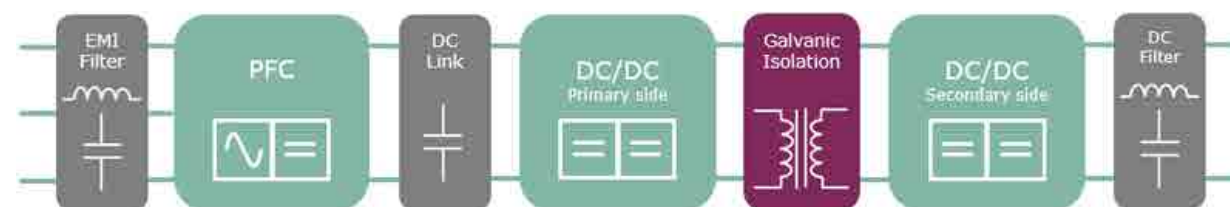
Figure 1: Typical topology for charging sub-unit in 15 – 40 kW range
