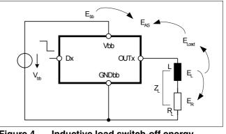
Figure 4 Inductive load switch-off energy dissipation (each channel)
