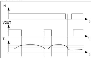
Figure 5 Overtemperature detection
