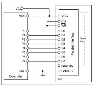
Figure 9 Parallel Direct Control
