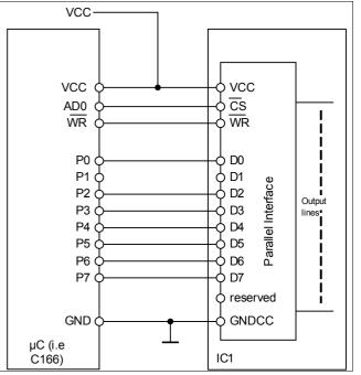
Figure 8 Parallel bus configuration
