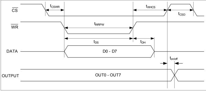
Figure 10 Parallel input - output timing diagram
