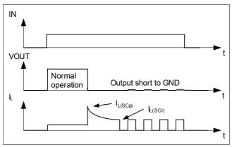
Figure 7 Short circuit in on-state, shut down down by overtemperature, restart by cooling
