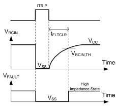
Figure 5: RCIN and FLT pin waveforms
