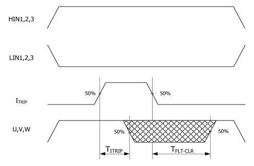
Figure 3: ITRIP Timing Waveform
