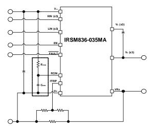
Figure 4b: Programming the fault clear timer
