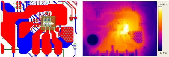
Figure 7: PCB layout example and corresponding thermal image
