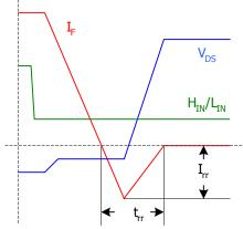
Figure 2c: Diode Reverse Recovery.
