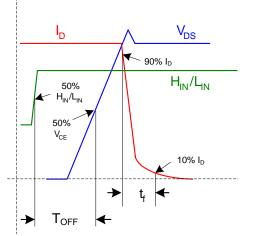
Figure 2b: Input to Output propagation turn-off delay time.
