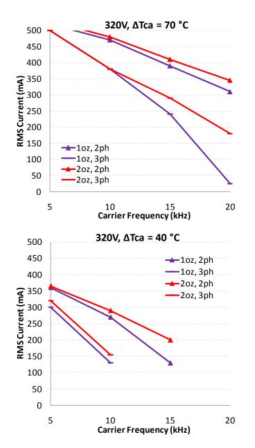
Figure 6: Maximum Sinusoidal Phase Current vs. PWM Switching Frequency Sinusoidal Modulation, V<sup>+</sup>=320V, PF=0.95
