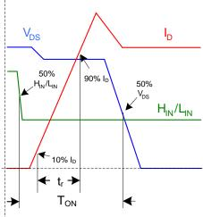
Figure 2a: Input to Output propagation turn-on delay time.
