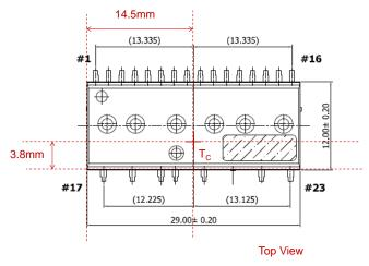
Figure 2: T<sub>C</sub> measurement point for R<sub>th(j-C)</sub>
