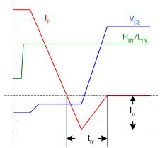
Figure 1c: Diode Reverse Recovery.
