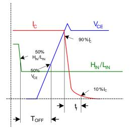
Figure 1a: Input to Output propagation turn-on delay time.
