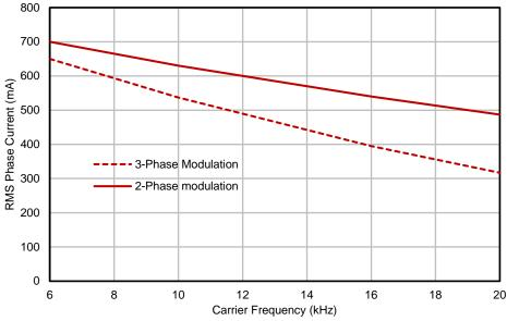
**Figure 6:** Maximum sinusoidal phase current vs PWM switching frequency, no heat sink. Space Vector Modulation, V+=320V, T<sub>A</sub>=28°C, T<sub>J</sub>=128°C
