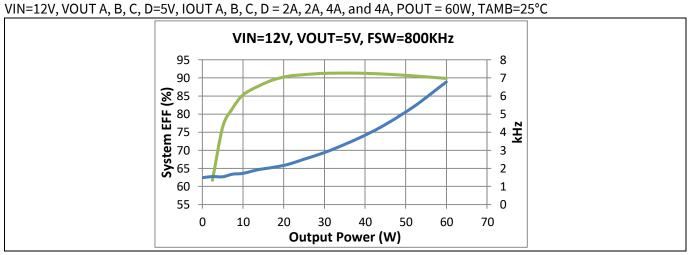
Figure 34 Total System Efficiency and power dissipation from 0W to 60W out
