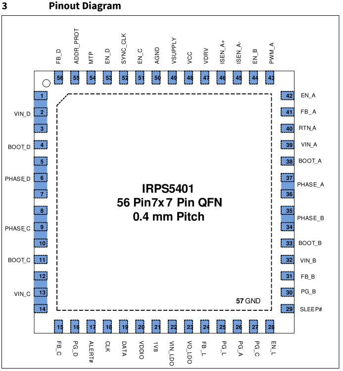
Pinout diagram 7mm x 7mm QFN (Top View) Figure 3
