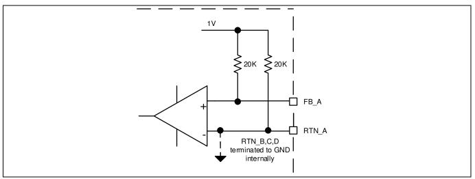
Figure 12 Output Voltage Sensing impedance
