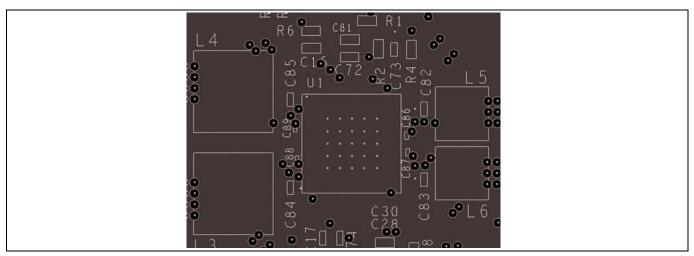
Figure 22 LAYER 3 – Signal Layer
