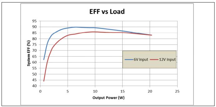
Figure 2 System efficiency with VO= 2.5V, FSW=800kHz, Tj=45°C
