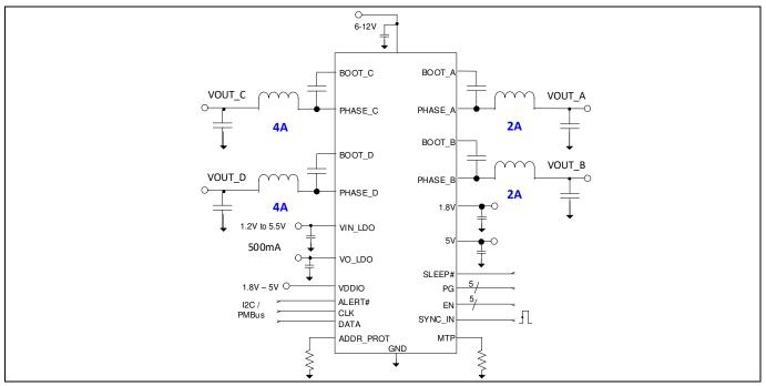
Figure 1 IRPS5401 Basic application circuit
