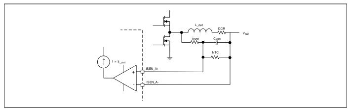
Figure 15 DCR Current Sensing
