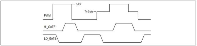
Figure 10 PWM\_A tri-state details
