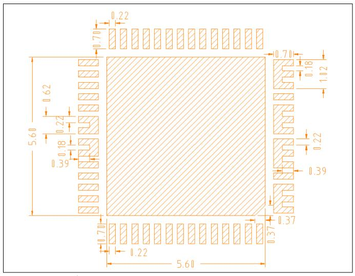
Figure 39 **PCB PAD Size**
