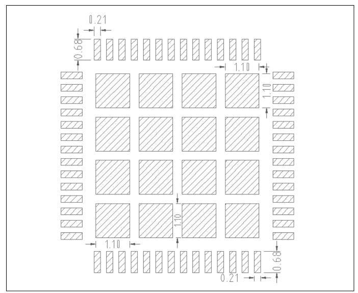
Figure 41 Solder paste stencil pad size
