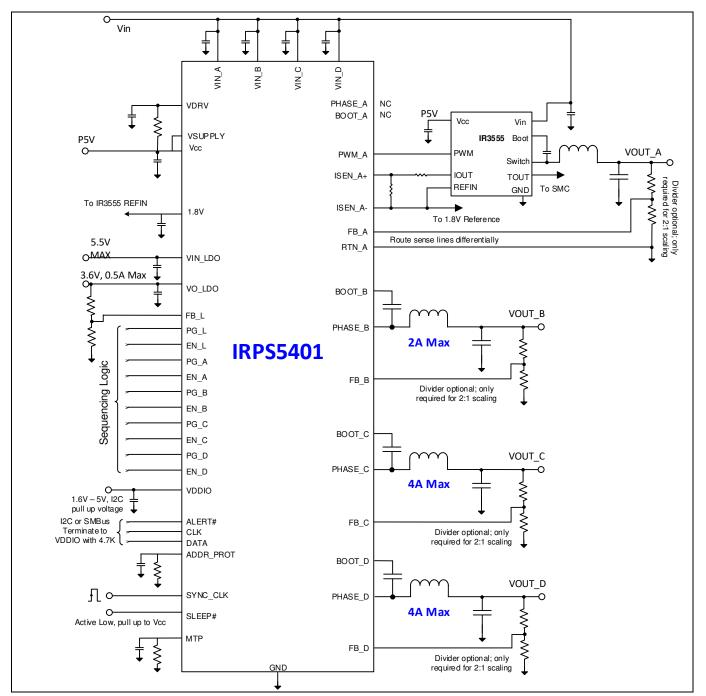
Figure 6 IRPS5401 using external IR MOSFET<sup>™</sup> Power Stage for high Current Output
