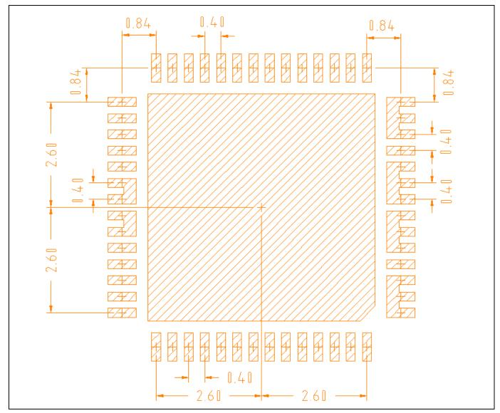
Figure 40 PCB PAD Spacing
