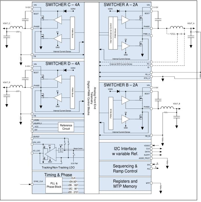
Figure 4 IRPS5401 Block Diagram
