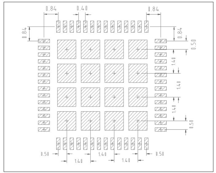
Figure 42 Solder paste stencil pad spacing
