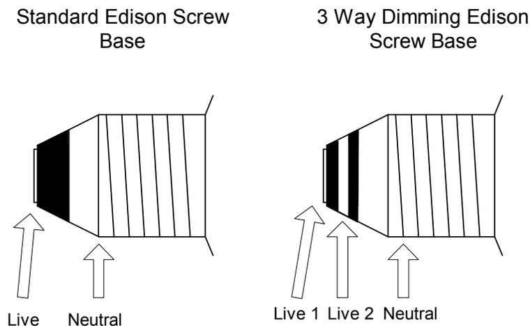
**Figure 2.1: Three way dimming Edison screw base**
