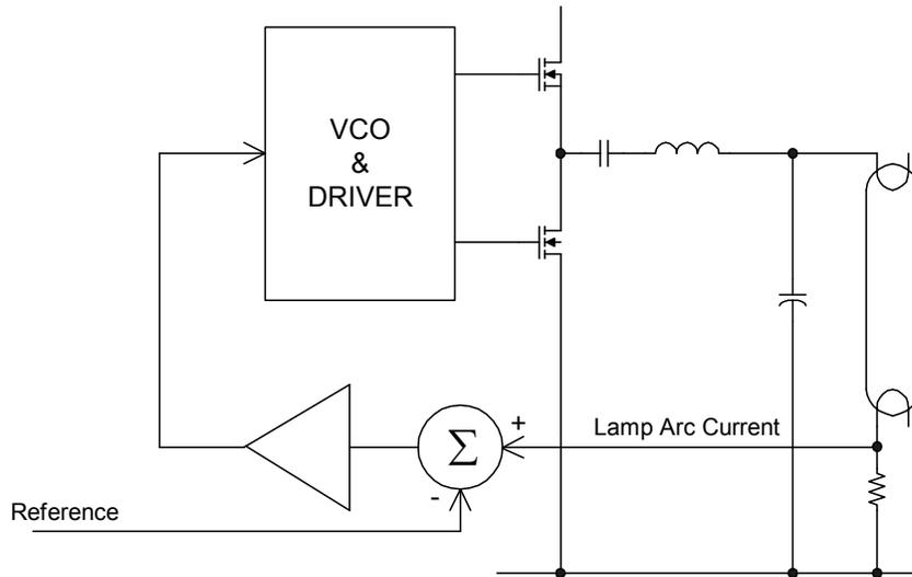
Figure 2.4: Closed loop lamp arc current regulation
