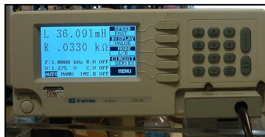
Figure 2—Measuring the Q phase and D phase Inductances.
