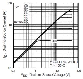
Fig 2. Typical Output Characteristics
