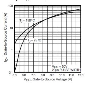
Fig 3. Typical Transfer Characteristics
