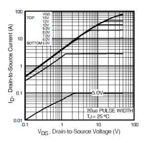
Fig 1. Typical Output Characteristics
