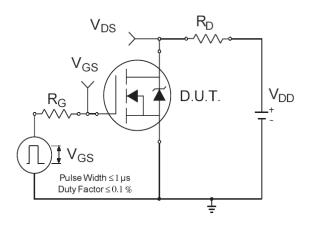
Fig 14a. Switching Time Test Circuit
