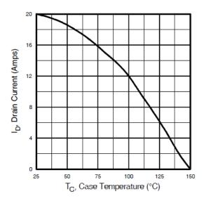
Fig 9. Maximum Drain Current Vs.Case
