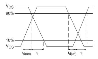
Fig 14b. Switching Time Waveforms
