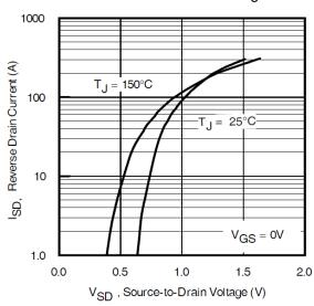
Fig 11. Typical Source-Drain Diode Forward Voltage
