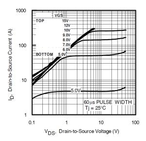
Fig 1. Typical Output Characteristics
