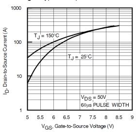
Fig 3. Typical Transfer Characteristics
