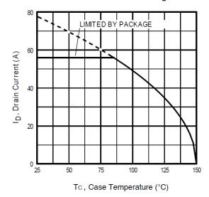
Fig 12. Maximum Drain Current Vs.Case Temperature
