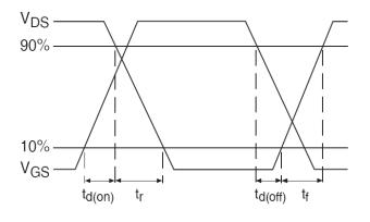
Fig 18b. Switching Time Waveforms
