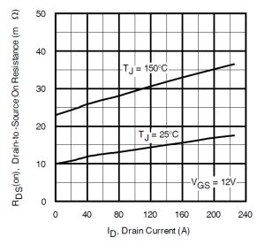
Fig 6. Typical On-Resistance Vs Drain Current
