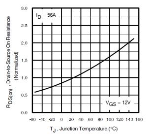
**Fig 4.** Normalized On-Resistance Vs. Temperature
