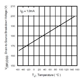
**Fig 7.** Typical Drain-to-Source Breakdown Voltage Vs Temperature
