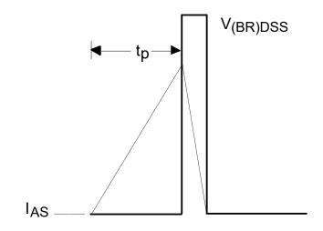
Fig 16b. Unclamped Inductive Wave-
