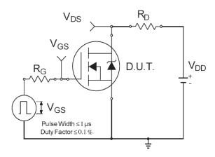
Fig 18a. Switching Time Test Circuit
