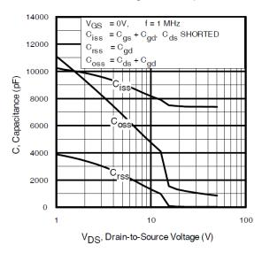
**Fig 9.** Typical Capacitance Vs. Drain-to-Source Voltage
