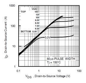
Fig 2. Typical Output Characteristics
