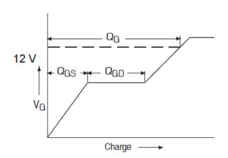
Fig 17a. Gate Charge Waveform
