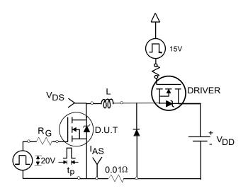
Fig 16a. Unclamped Inductive Test Circuit
