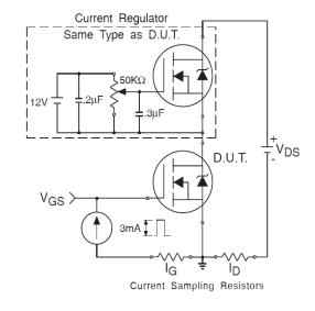
Fig 17b. Gate Charge Test Circuit
