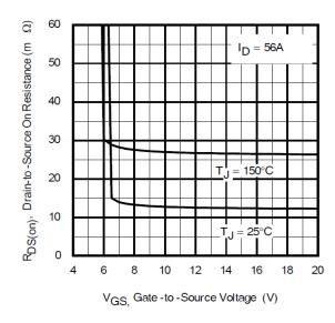
Fig 5. Typical On-Resistance Vs Gate Voltage
