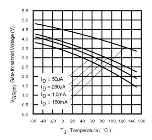
**Fig 8.** Typical Threshold Voltage Vs Temperature
