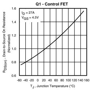
Fig 13. Normalized On-Resistance vs. Temperature
