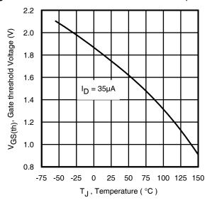
Fig 21. Threshold Voltage vs. Temperature
