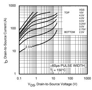
Fig 4. Typical Output Characteristics
