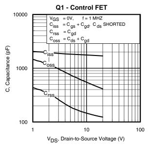
Fig 7. Typical Capacitance vs. Drain-to-Source Voltage
