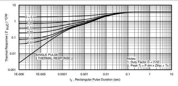
Fig 25. Maximum Effective Transient Thermal Impedance, Junction-to-Case (Q1)
