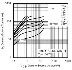
Fig 3. Typical Output Characteristics
