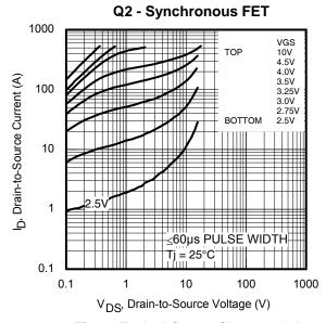
Fig 2. Typical Output Characteristics
