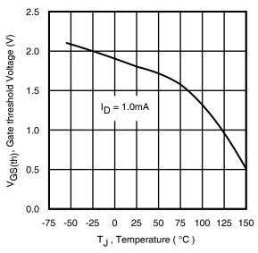
Fig 22. Threshold Voltage vs. Temperature
