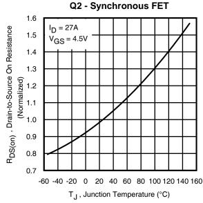
Fig 14. Normalized On-Resistance vs. Temperature
