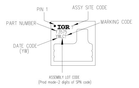
Figure 6: PQFN 6mm x 6mm
