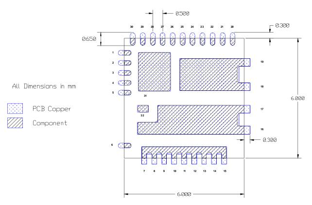
Figure 3: Metal and component placement
