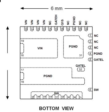
Figure 1: IRF3575DPbF Bottom View
