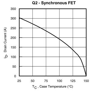
Fig 20. Maximum Drain Current vs. Case Temperature
