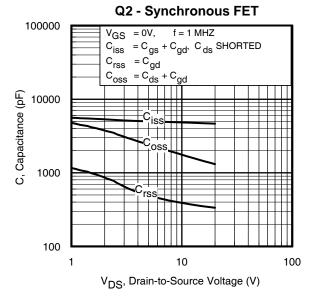
Fig 8. Typical Capacitance vs. Drain-to-Source Voltage
