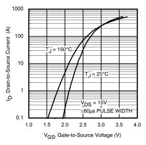
Fig 6. Typical Transfer Characteristics
