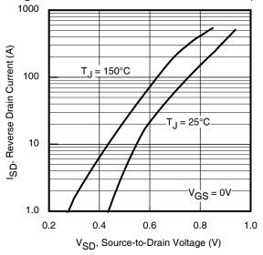
Fig 16. Typical Source-Drain Diode Forward Voltage
