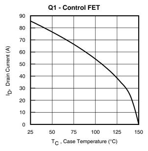
Fig 19. Maximum Drain Current vs. Case Temperature
