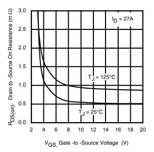
Fig 18. Typical On-Resistance vs. Gate Voltage
