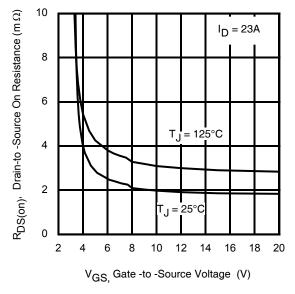
Fig 17. Typical On-Resistance vs. Gate Voltage
