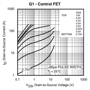
Fig 1. Typical Output Characteristics
