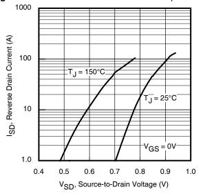
Fig 15. Typical Source-Drain Diode Forward Voltage
