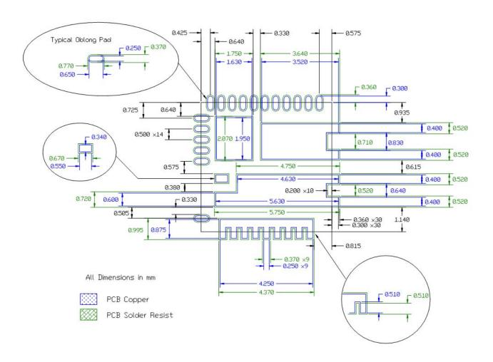
Figure 4: Solder resist
