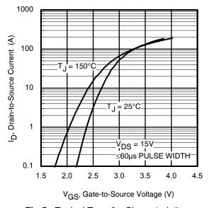
Fig 5. Typical Transfer Characteristics
