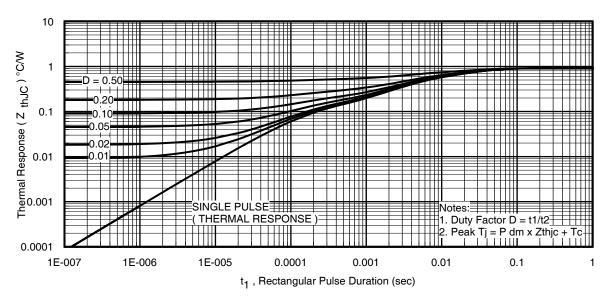
Fig 26. Maximum Effective Transient Thermal Impedance, Junction-to-Case (Q2)
