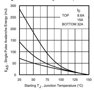
Fig 23. Maximum Avalanche Energy vs. Drain Current
