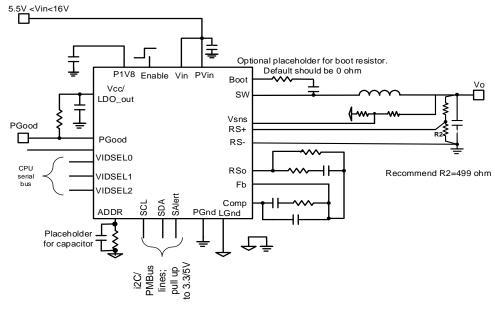
Figure 5: Using the internal LDO, Vo > 2.555V
