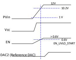
Figure 9: Normal Start up, device turns on when the bus voltage reaches 10.2A. A resistor divider is used at EN pin from PVin to turn on the device at 10.2V.
