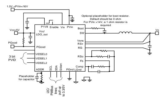
Figure 6: Using external Vcc, Vo<2.555V
