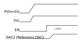
Figure 10: Recommended startup for Normal operation
