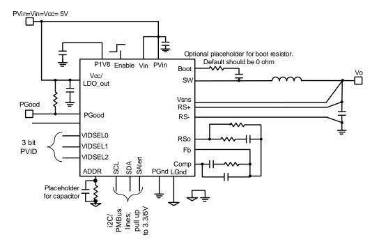
Figure 7: Single 5V application, Vo<2.555V
