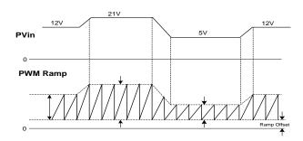
Figure 17: Timing Diagram for Feed-Forward (F.F.) Function
