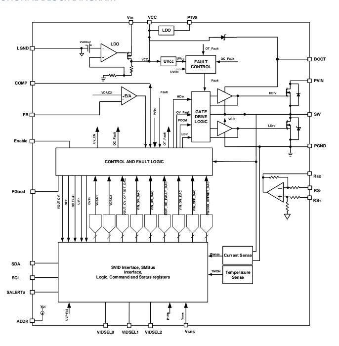
Figure 3: Simplified Block Diagram for IR38263
