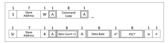
Figure 28: SMBus Block Read with Byte Count=1
