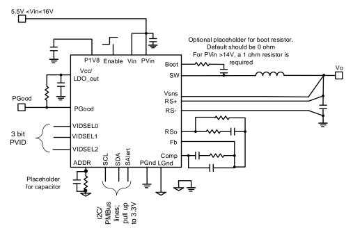
Figure 4: Using the internal LDO, Vo < 2.555V
