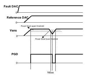
Figure 19: Power Good in PMBus™ mode
