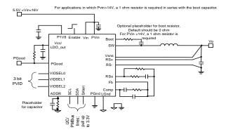
Figure 1: Typical application circuit
