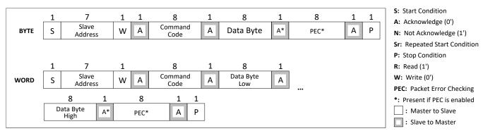
Figure 25: SMBus Write Byte/Word
