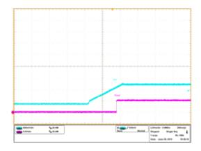
Figure 47: 0.35V Prebias voltage startup at 0A load  ${\rm Ch_2:V_{out},\,Ch_3:P_{Good}}$
