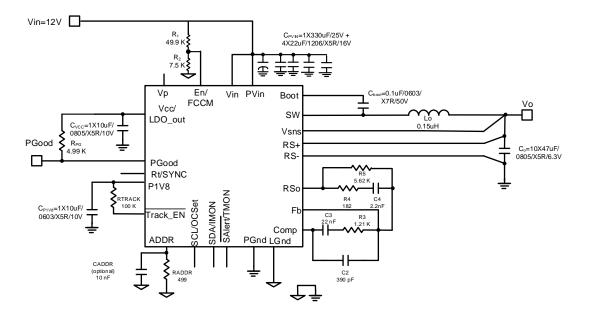
Figure 40: Application circuit for a single supply, 12V to 1.2V, 35A Point of Load Converter
