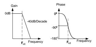
Figure 37: Gain and Phase of LC filter
