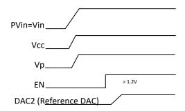
Figure 13: Recommended startup for Normal operation
