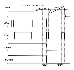
Figure 32: Timing Diagram for OVP in nontracking mode
