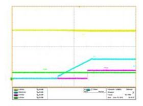
$\label{eq:Figure 43:Operation 80,Turn ON without margining, 35A load \\ \text{Ch}_{\text{1}:P}_{\text{Vin}}, \text{Ch}_{\text{2}:V}_{\text{out}}, \text{Ch}_{\text{3}:P}_{\text{Good}}, \text{Ch}_{\text{4}:Enable}$
