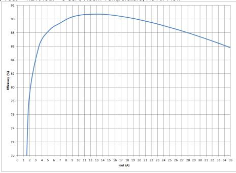
Figure 53: Efficiency versus load current
