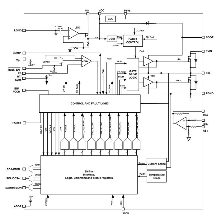
Figure 4: IR38064 Simplified Block Diagram
