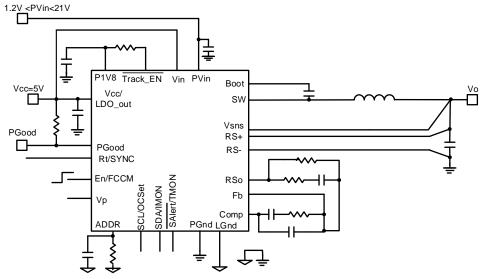
Figure 8: Using external Vcc, digital mode, Vo<2.555V
