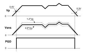
Figure 30: Vp Tracking (Track\_En = 0V)
