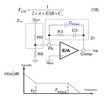
Figure 38: Type II compensation network and its asymptotic gain plot
