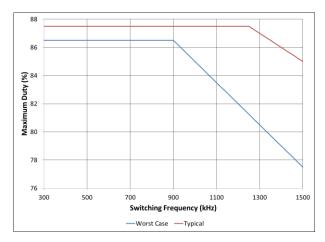
Figure 33: Maximum duty cycle vs. switching frequency
