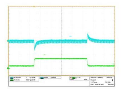
Figure 49: Transient Response, 3.5A to 14A step (2.5A/us)  ${\rm Ch_1:V_{out},\,Ch_4:I_{out}}$
