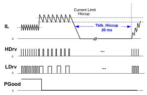
Figure 21: Timing Diagram for Current Limit Hiccup
