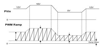
Figure 24: Timing Diagram for Feed-Forward (F.F.) Function
