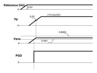
Figure 31: Vp Sequencing (100 kOhm from Track\_En to P1V8)
