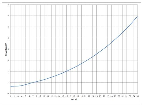
Figure 54: Power loss versus load current
