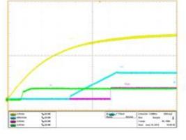
Figure 42:PV<sub>in</sub> Start up at 35A Load Ch<sub>1</sub>:P<sub>Vin</sub>, Ch<sub>2</sub>:V<sub>out</sub>, Ch<sub>3</sub>:P<sub>Good</sub>,Ch<sub>4</sub>:V<sub>cc</sub>
