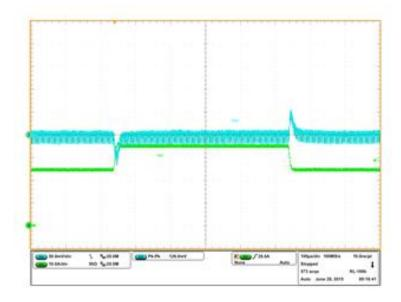
Figure 50: Transient Response, 24.5A to 35A step (2.5A/us)  $\mathrm{Ch_1:V_{out},\,Ch_4:I_{out}}$
