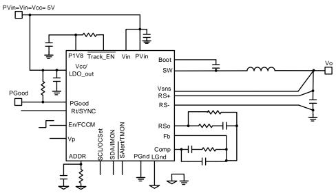
Figure 9: Single 5V application, digital mode, Vo<2.555V
