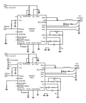
Figure 26: Application Circuit for Simultaneous and Ratiometric Sequencing of two Manhattan devices
