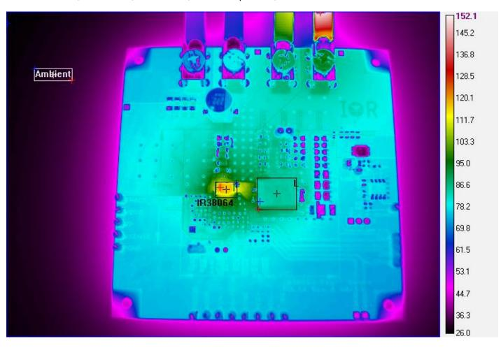
Figure 55: Thermal Image of the board at 35A load IR38064: 120.2°C, inductor: 89.89°C, Ambient:29.8°C
