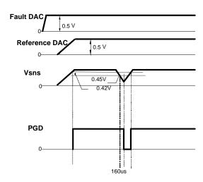
Figure 29: Non-sequenced, Non-tracking Startup
