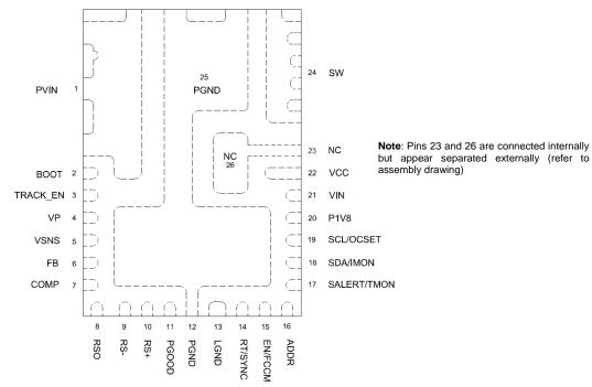
Figure 3: IR38064 package (Top View) 5mm x 7mm PQFN
