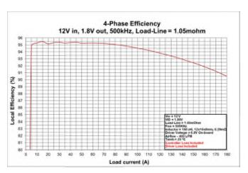
Figure 37: Light Load Efficiency Improvement with DPC
