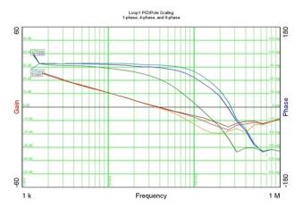
Figure 28: Stability with Phase Add/Drop
