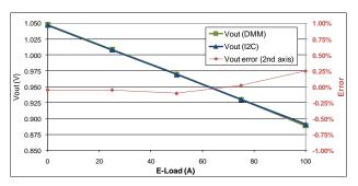
Figure 47: I2C Output Voltage Measurements
