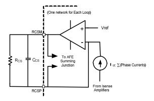
Figure 26 Load Line for RDS (ON) Current Sense
