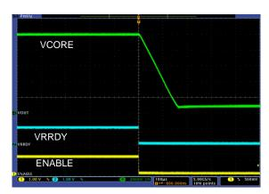
Figure 12: Enable-based Shutdown
