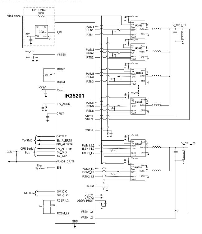
Figure 3: VR using IR35201 Controller and IR3555 PowIR Stage in 6+2 Configuration
