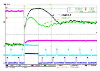
Figure 31: Diode Emulation during a load release
