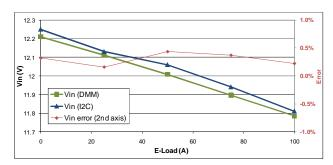
Figure 46: I2C Input Voltage Measurements
