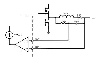
Figure 21: DCR Current Sensing
