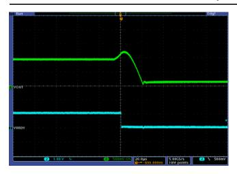
Figure 41: OVP - MOSFET released when output<0.3V
