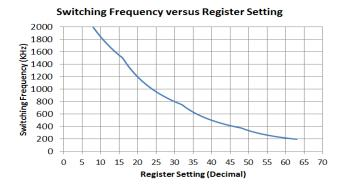
Figure 17: Switching Frequency Variation with Register Setting
