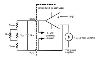
Figure 25: Load Line & Thermal Compensation for DCR Sense
