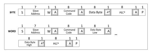
Figure 54: PMBus Write Byte/Word
