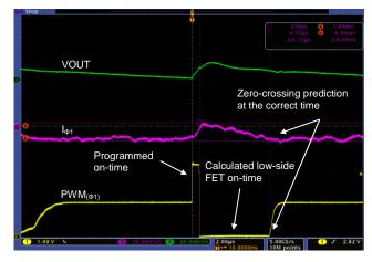
Figure 39: PS2 Active Diode Emulation Mode
