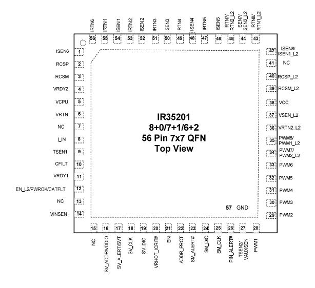
Figure 1: IR35201 Pin Diagram
