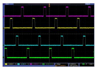
Figure 16: 4-phase PWM interleaved operation
