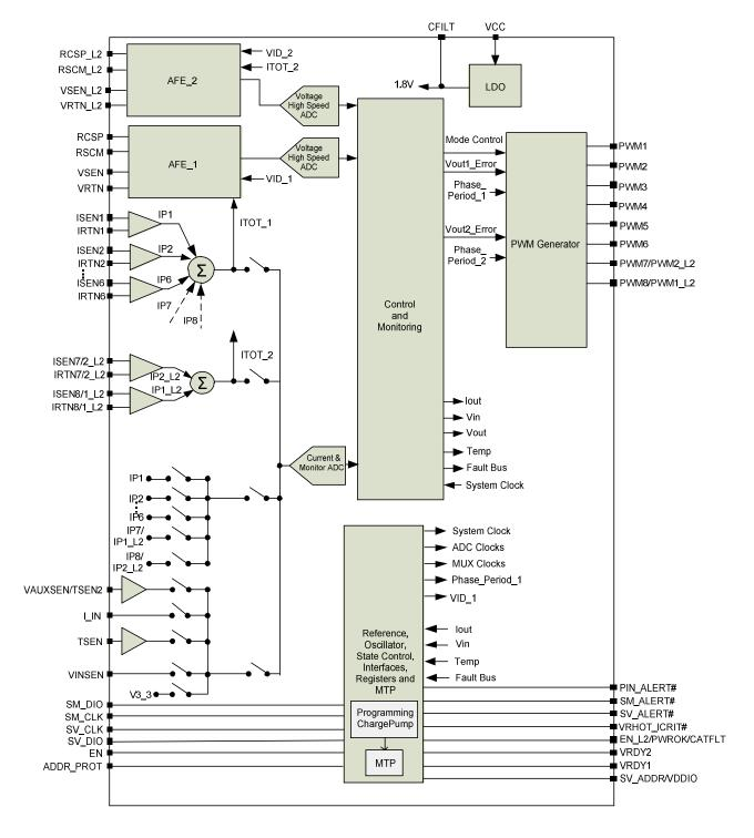
Figure 2: IR35201 Block Diagram
