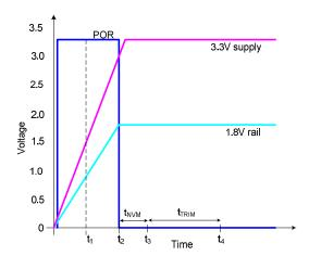
Figure 6: Controller Startup and Initialization
