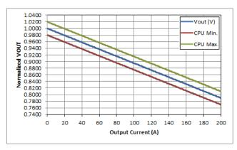
Figure 27: Load Line Measurements
