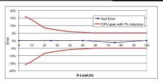
Figure 45: I2C I<sub>OUT</sub> Error using 10% DCR Inductors
