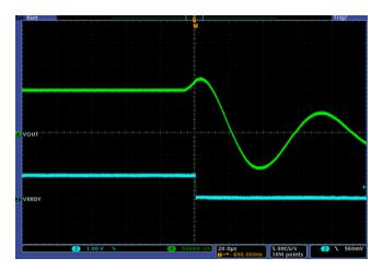
Figure 40: OVP - MOSFET latched on
