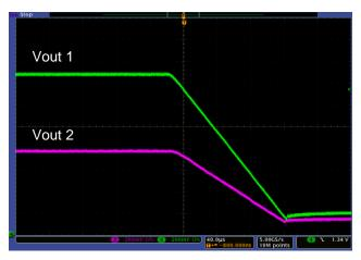
Figure 15: MPoL Tracking Shutdown
