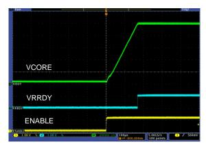
Figure 11: Enable-based Startup
