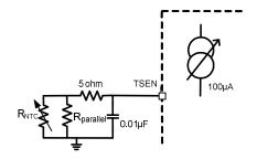
Figure 42: Temperature Sense NTC Network
