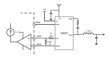
Figure 22 R<sub>DS (ON)</sub> Current Sense
