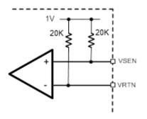
Figure 19: Output Voltage sensing impedance
