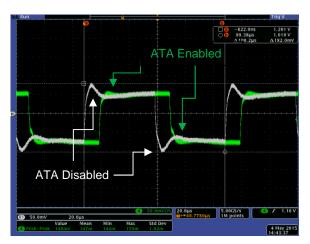
Figure 29: ATA Enable/Disable Comparison
