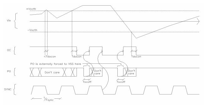
Figure 4: OC timing diagram
