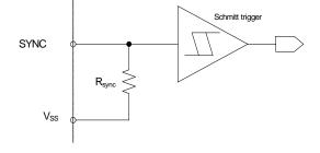
Figure 2: Sync input circuit
