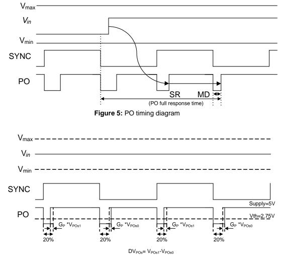
Figure 6: ∆offset between two consecutive samples measured at PO
