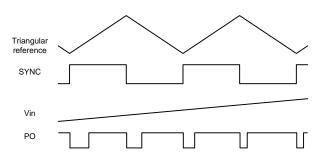
Figure 10: Main current sensor signals and outputs
