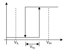
Figure 1: Sync input thresholds
