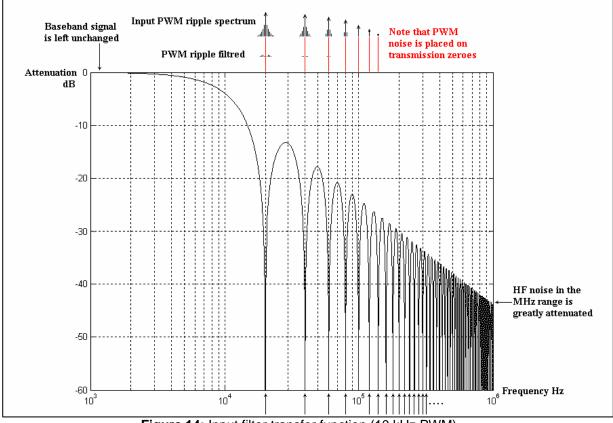
Figure 14: Input filter transfer function (10 kHz PWM)
