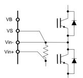
Figure 18: Recommended shunt connection
