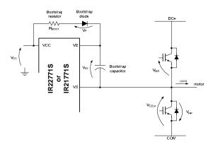
Figure 16: bootstrap supply schematic
