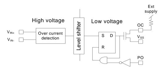
Figure 9: Over current block diagram
