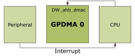
Hardware triggered transfers or asynchronous transfers make use of the service request signals of the peripheral to initiate the DMA transaction. DMA acts as flow controller
