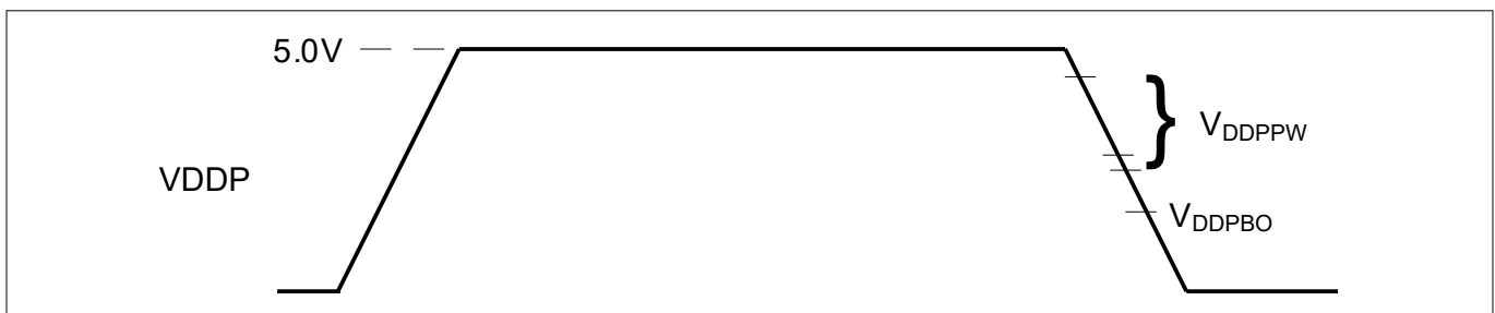
Figure 17 Supply Threshold Parameters
