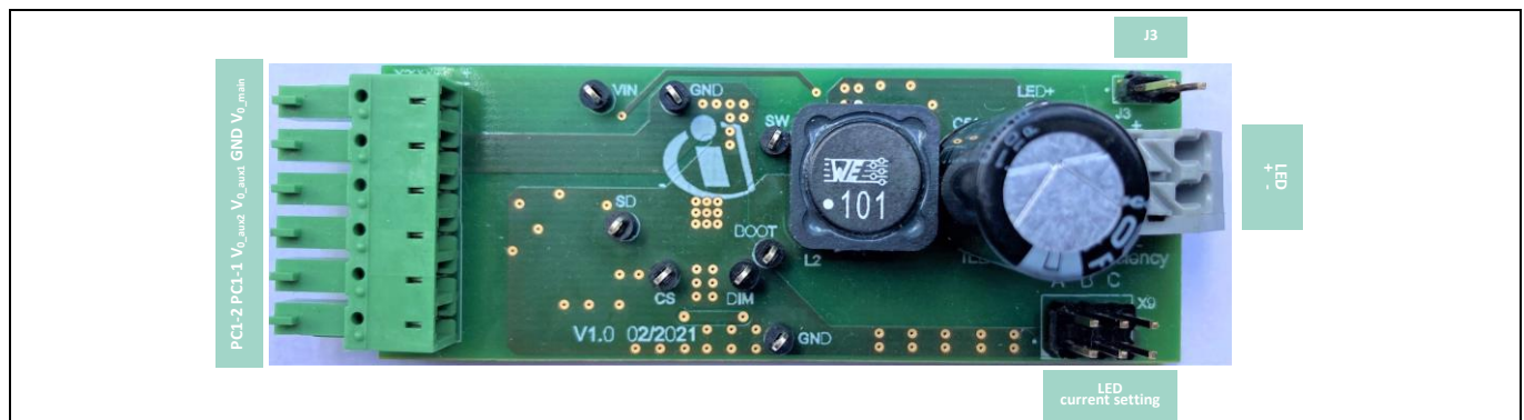
Figure 7 Reference design – dimensions 81 mm (L) x 27 mm (W) x 24 mm (H)
