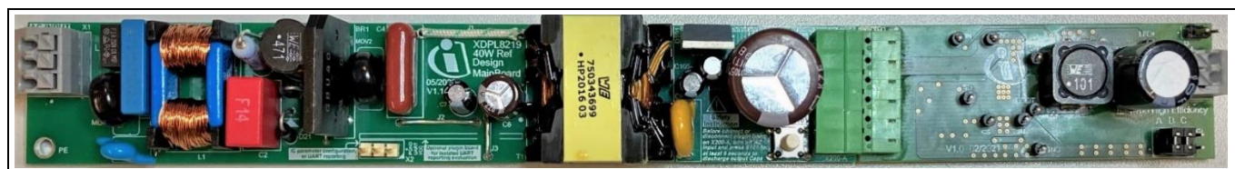
Figure 9 System XDPL8219 reference design + ILD8150_HE board
