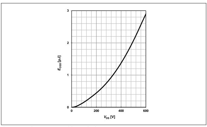
Figure 4 Typical output energy (single switch)
