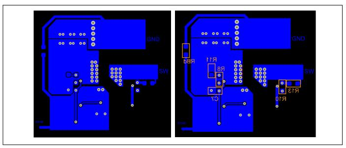
Figure 15 Bottom layer of the PCB - top view (Trace on the left and silk mask on the right)
