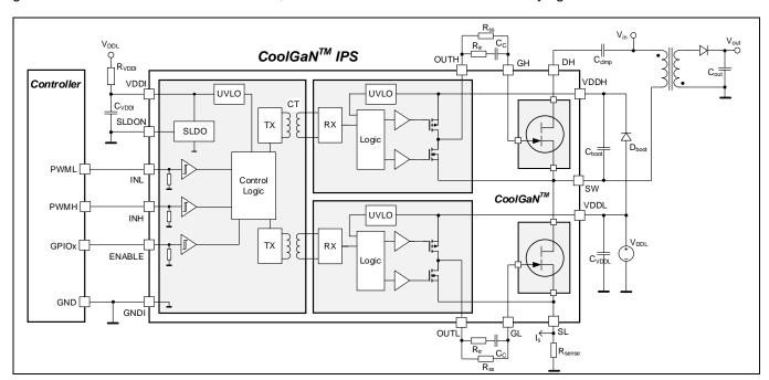
Figure 1 Typical application circuit (active clamp flyback converter)
