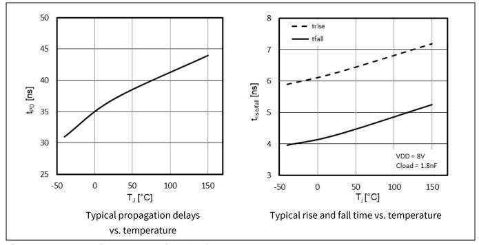
Figure 9 Propagation delay and rise / fall times
