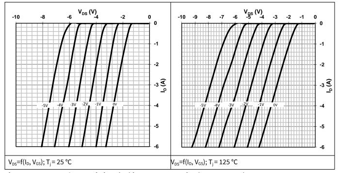
Figure 1 Output characteristic I<sub>ds</sub> (V<sub>ds</sub>) in reverse operation (parameter V<sub>gs</sub>)
