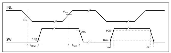
Figure 4 Propagation delay, rise and fall time
