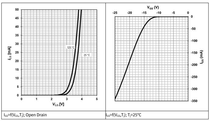
Figure 11 Typical gate characteristics forward and reverse
