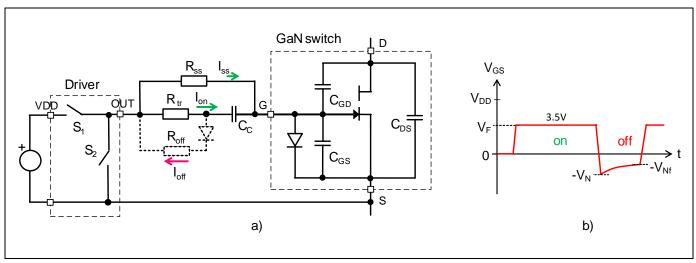
Figure 8 Equivalent circuit of GaN switch with RC gate drive (a) and gate-to-source voltage V<sub>GS</sub> (b)
