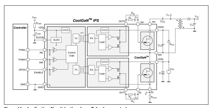
Figure 10 Application Circuit (active clamp flyback converter)
