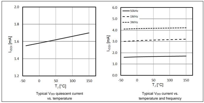
Figure 5 Supply current V<sub>DDI</sub>
