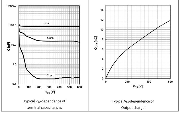
Figure 3 Terminal capacitances and output charge (single switch)
