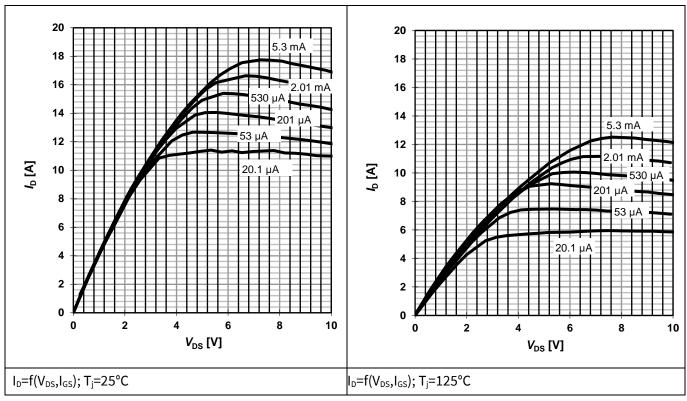
Figure 9 Typical output characteristics
