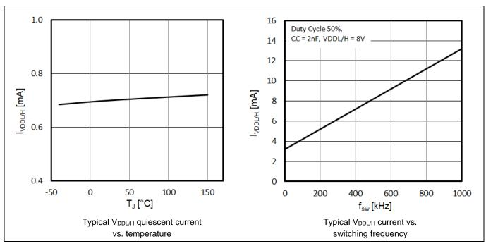
Figure 6 Supply current V<sub>DDL/H</sub>
