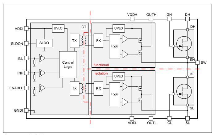
Figure 3 Block Diagram IGI60F2727A1L
