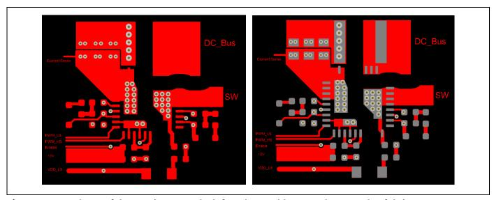
Figure 14 Top layer of the PCB (trace on the left and top solder paste layer on the right)
