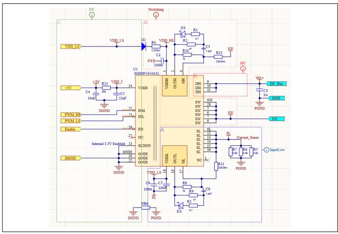
Figure 13 CoolGaN™ IPS circuitry with external passive components
