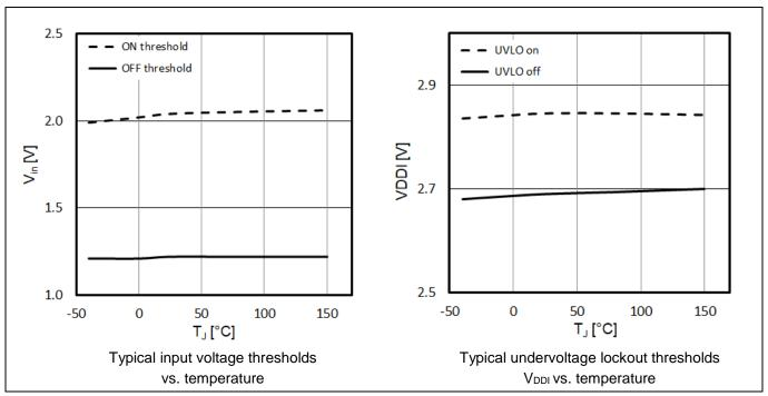
Figure 7 Logic input thresholds and V<sub>DDI</sub> UVLO
