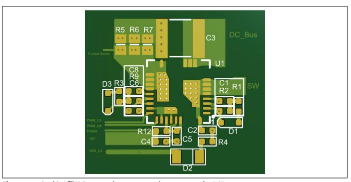
Figure 12 CoolGaN™ IPS external component placement on the PCB
