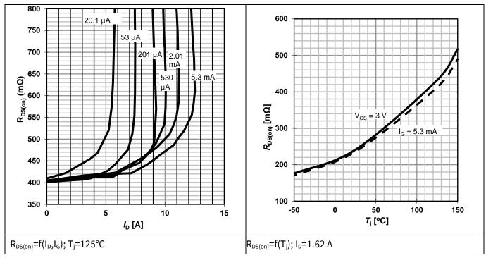
Figure 10 Typical drain-source on-resistance
