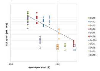
Figure 6: EOL cycles for the tested devices depending on current per bond. The measured cycles were normalized to  $T_{jmean}$  = 105°C,  $\Delta T$  = 90°C. Points indicate devices with heel crack as EOL fail mode, open squares indicate DUTs with bond lift-off as EOL fail mode
