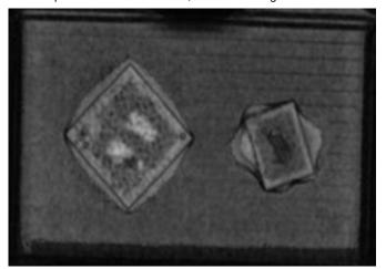
Figure 3: SAM picture of chip, front side: Non-disturbed bond wire foot remains black for the diode; the complete bright area for the upper IGBT bond wire foot indicates bond wire lift-off. This is in confirmed after removal of the mold compound (decap), Figure 4
