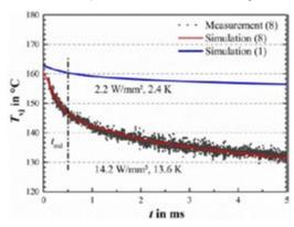
Figure 2: FEM simulation of temperature progression after pulse switch-off; simulation matches very well with measurements as shown for DUT8
