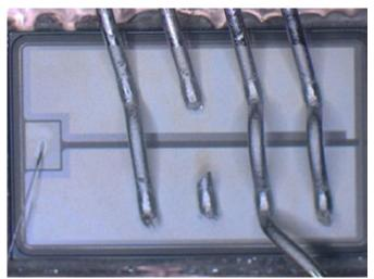
Figure 5: Heel crack of bond wires after power-cycling
