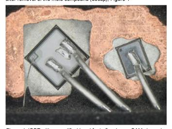
Figure 4: IGBT with upper lifted bond foot after decap, SAM showed complete bright area for this bond foot
