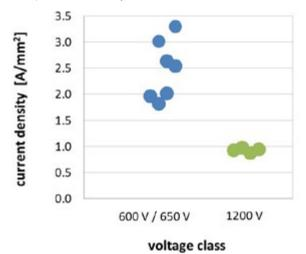
Figure 8: Current per device area, current density, grouped by voltage class
