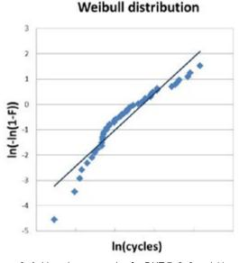
Figure 9: Achieved power cycles for DUT 7, 8, 9 and 11
