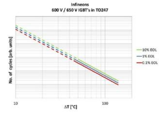
Figure 10: Achievable power cycles per  $\Delta T$  for 10%, 1% and 0.1% EOL. Curves are valid for pulse durations < 10 s and  $T_{jmean}$  = 80°C. Dashed lines indicate data extrapolation; solid lines are based on measured data
