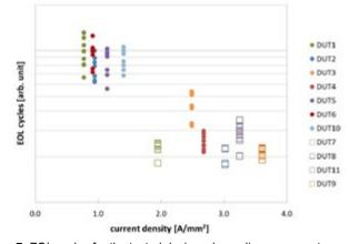
Figure 7: EOL cycles for the tested devices depending on current density
