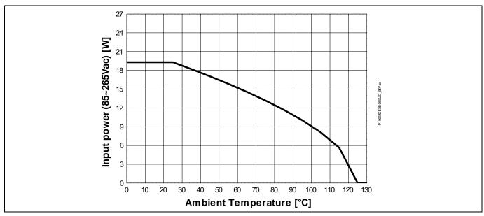
Figure 32 Input power curve V<sub>IN</sub>=85~265 V<sub>AC</sub>; P<sub>in</sub>=f(T<sub>a</sub>)
