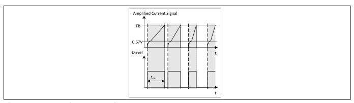
Figure 6 Pulse Width Modulation
