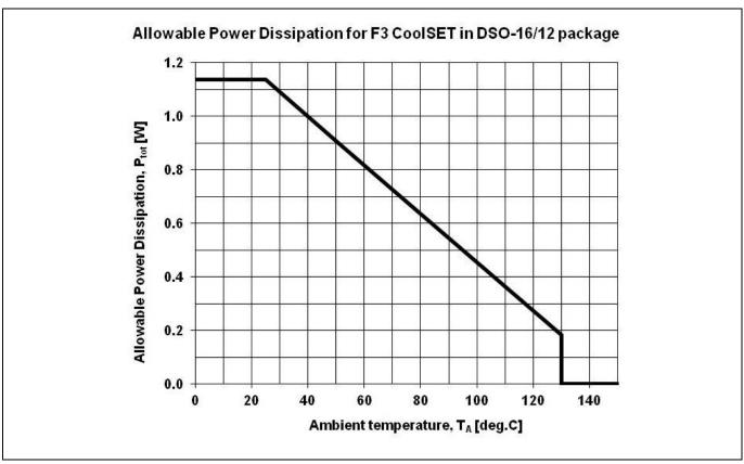
Figure 30 Power dissipation; Ptot=f(Ta)
