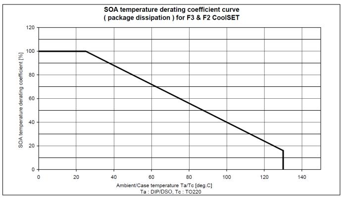
Figure 29 SOA temperature derating coefficient curve
