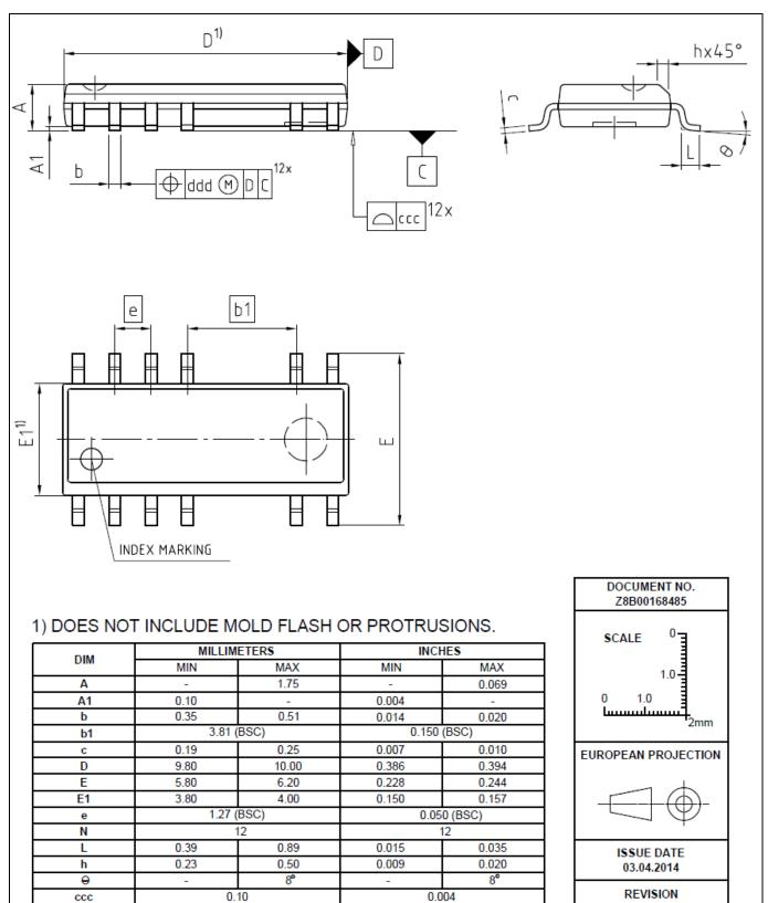
PG-DSO-12 (Pb-free lead plating Plastic Dual-in-Line Outline) Figure 34
