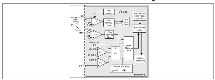
Figure 27 Over load, open loop protection
