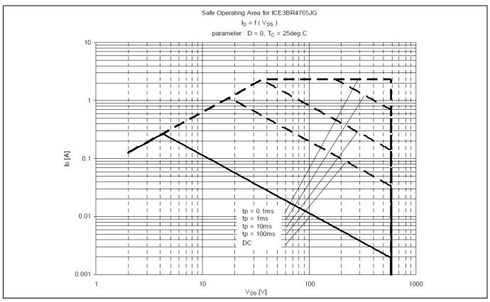
Figure 28 Safe Operating Area (SOA) curve for ICE3BR4765JG
