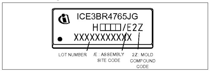
Figure 35 Marking for ICE3BR4765JG
