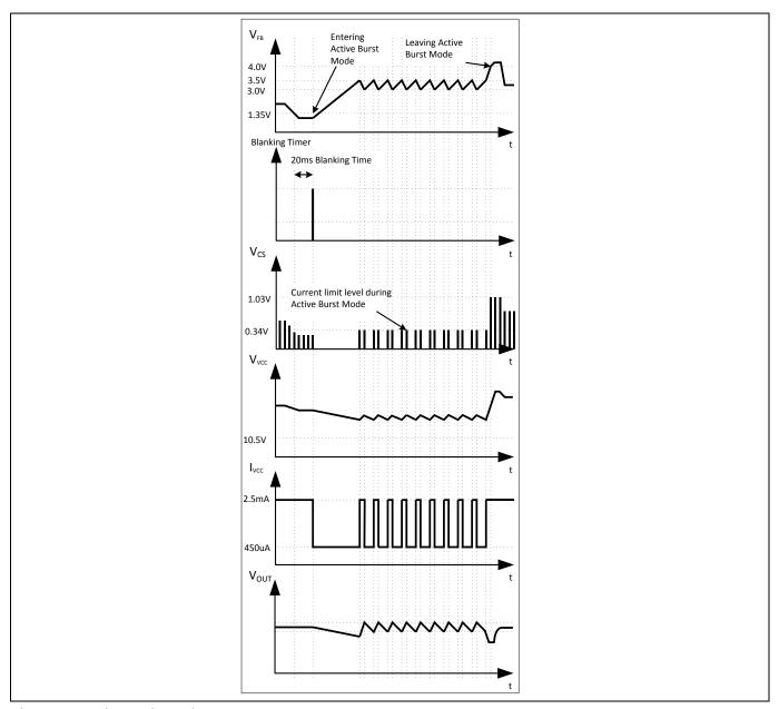
Figure 25 Signals in Active Burst Mode
