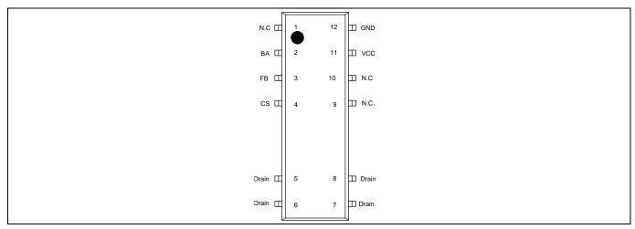
Figure 2 Pin configuration PG-DSO-12(top view)
