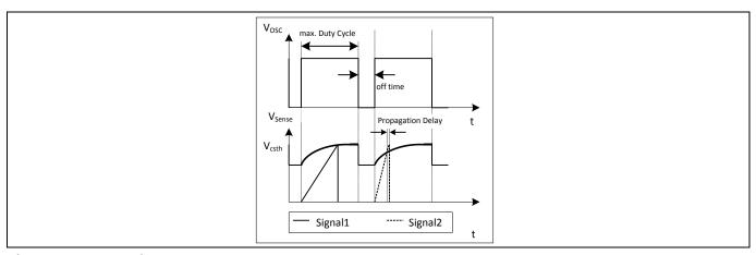
Figure 22 Dynamic Voltage Threshold V<sub>csth</sub>
