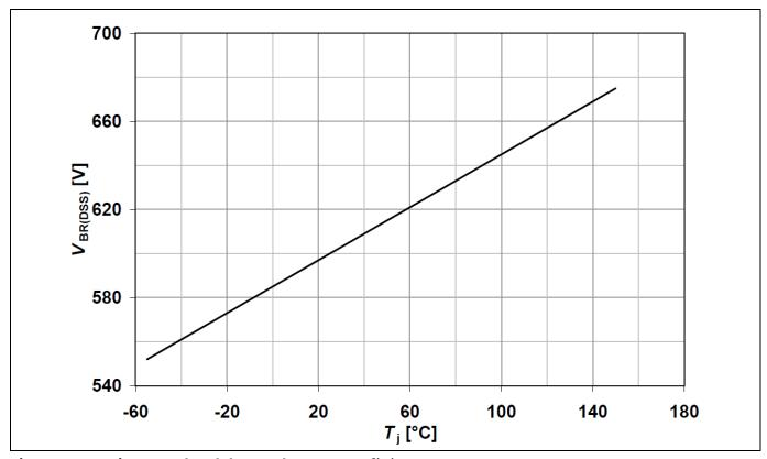
Figure 31 Drain-source breakdown voltage; V<sub>BR(DSS)=</sub> f(T<sub>j</sub>), I<sub>D</sub>=0.25mA
