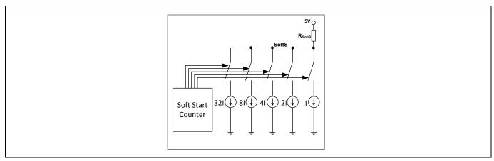
Figure 12 Soft Start Circuit
