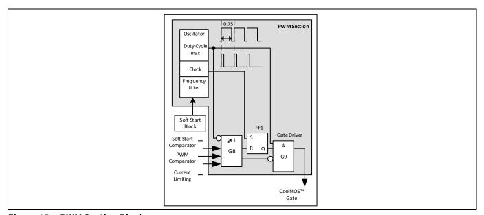
Figure 15 PWM Section Block
