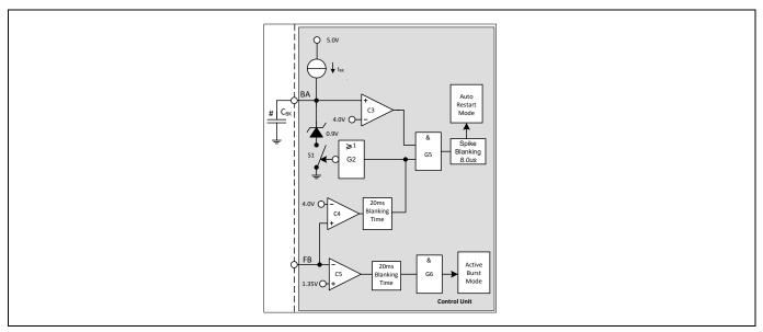
Figure 23 Basic and Extendable Blanking Mode
