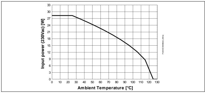
Figure 33 Input power curve V<sub>IN</sub>=230 V<sub>AC</sub>; P<sub>in</sub>=f(T<sub>a</sub>)
