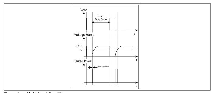
Figure 8 Light Load Conditions
