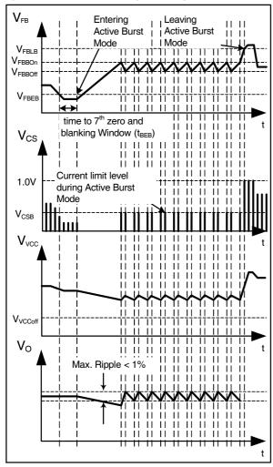
Figure 8 Signals in Active Burst Mode
