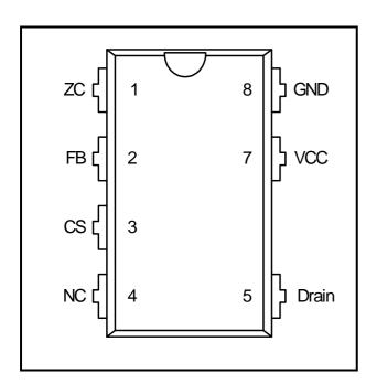
Figure 1 Pin Configuration PG-DIP7 (top view)
