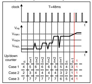
Figure 5 Up/down counter operation
