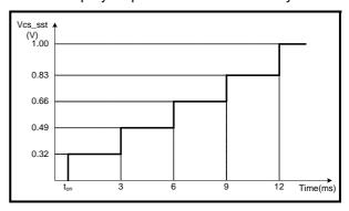
Figure 4 Maximum current sense voltage during softstart
