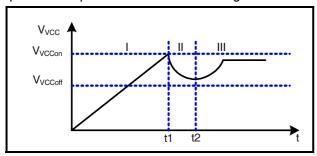
Figure 3 VCC voltage at start up
