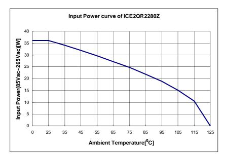
Figure 12 Input Power curve  $Vin=230Vac;Pin=f(T_a)$
