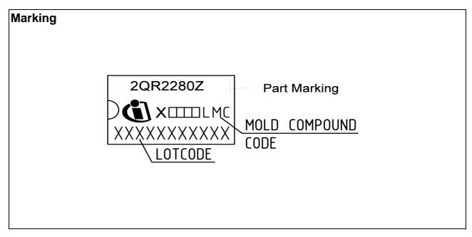
Figure 14 Marking for ICE2QR2280Z
