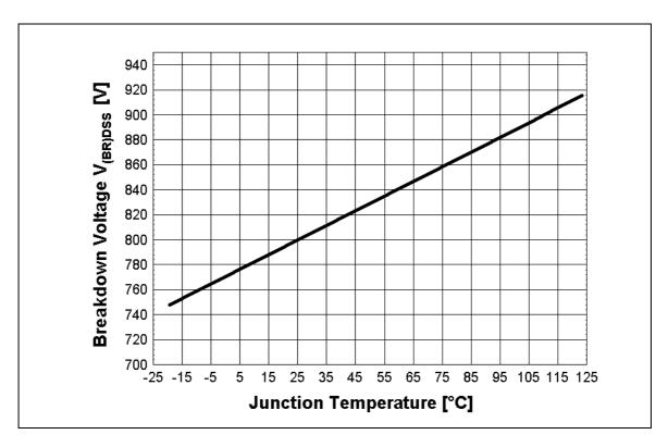
Figure 9 Drain-Source Breakdown voltage;  $V_{BR(DSS)} = f(T_j), I_D = 0.25 \text{mA}$
