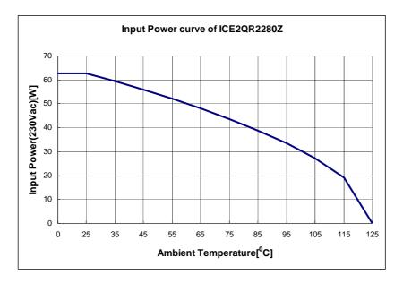
Figure 11 Input Power curve Vin=85~265Vac;Pin=f(T<sub>a</sub>)
