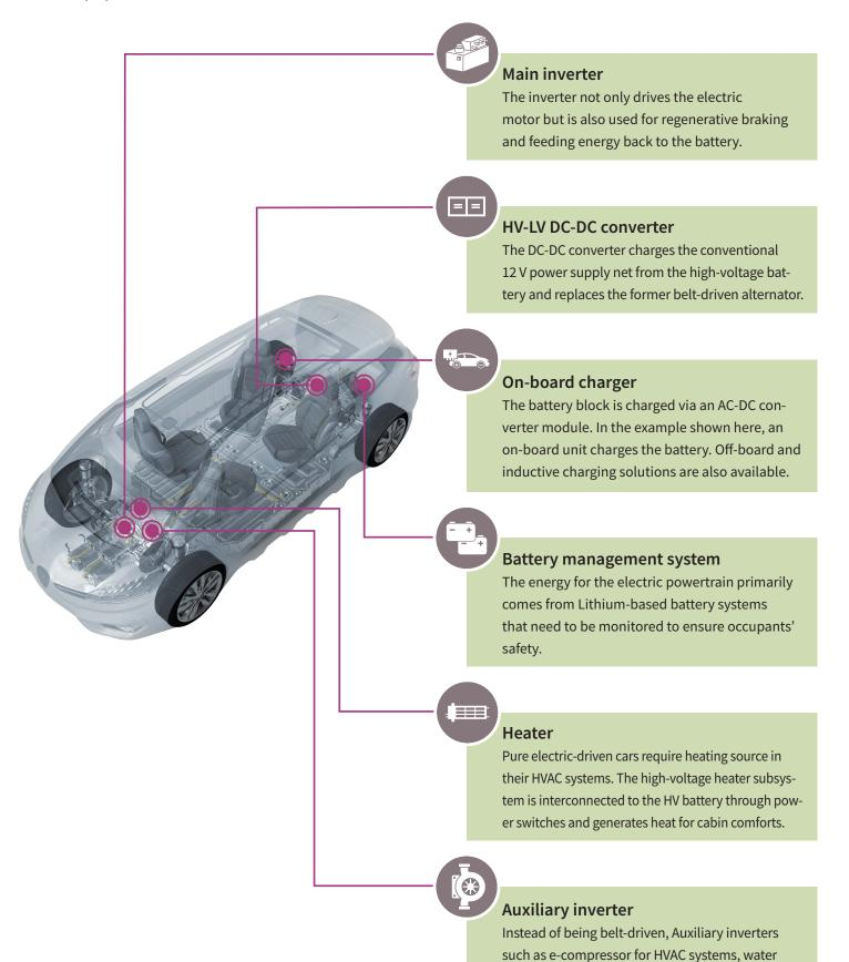
pumps, etc., are driven by electric power. Smart and energy-efficient auxiliary inverters are mainly realized through B6 bridges on its controller board.
