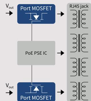
**Figure 2/3:** The PSE will require an efficient PFC and low-loss switches using an isolated topology (top), while PDs will make use of a generic DC/DC solution unless targeting specific applications such as LED lighting (bottom).
