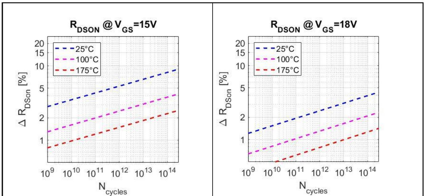
**Figure 8** Left: Relative  $R_{DS(on)}$  change at  $V_{GS(on)} = 15\text{ V}$ ,  $T_{vjop} = 25^\circ\text{C}$ ,  $100^\circ\text{C}$ , and  $175^\circ\text{C}$
