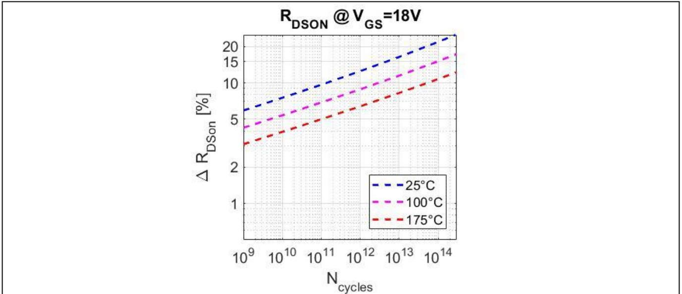
**Figure 6** Relative  $R_{DS(on)}$  change at  $V_{GS(on)} = 18\text{ V}$ ,  $T_{vjop} = 25^\circ\text{C}$ ,  $100^\circ\text{C}$ , and  $175^\circ\text{C}$  based on extrapolation of intermediate readouts
