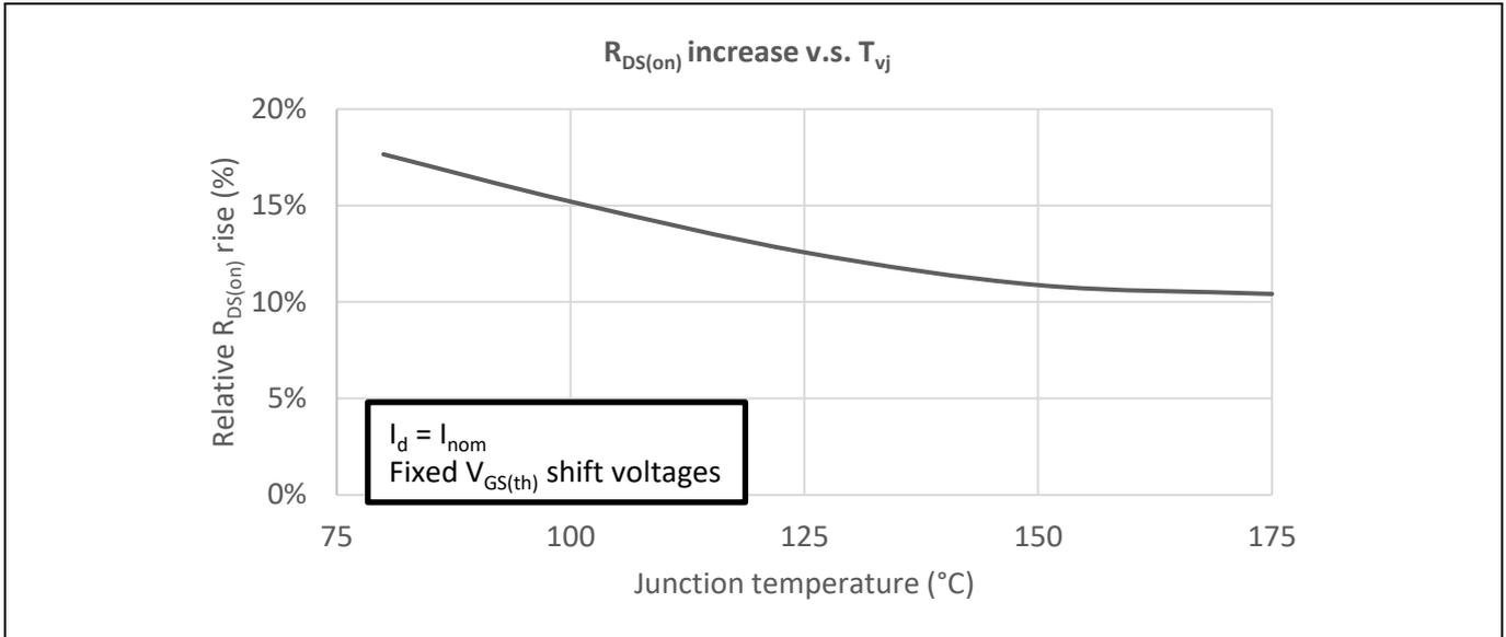
**Figure 4** Relative R<sub>DS(on)</sub> increase at different junction temperatures
