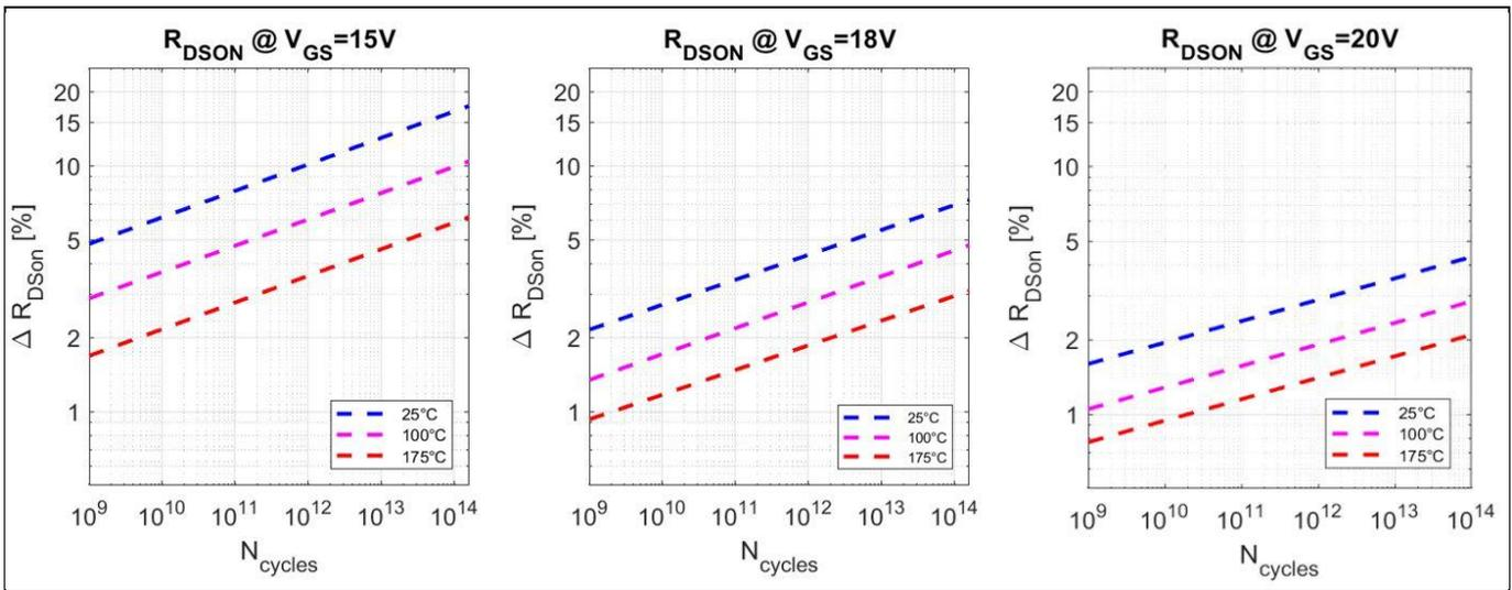
**Figure 5** Left: Relative  $R_{DS(on)}$  change at  $V_{GS(on)} = 15V$ ,  $T_{vjop} = 25^\circ C$ ,  $100^\circ C$ , and  $175^\circ C$
