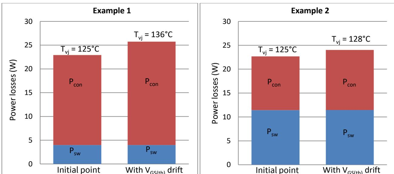
**Figure 1 Examples of  $V_{GS(th)}$  drift impact on applications**
