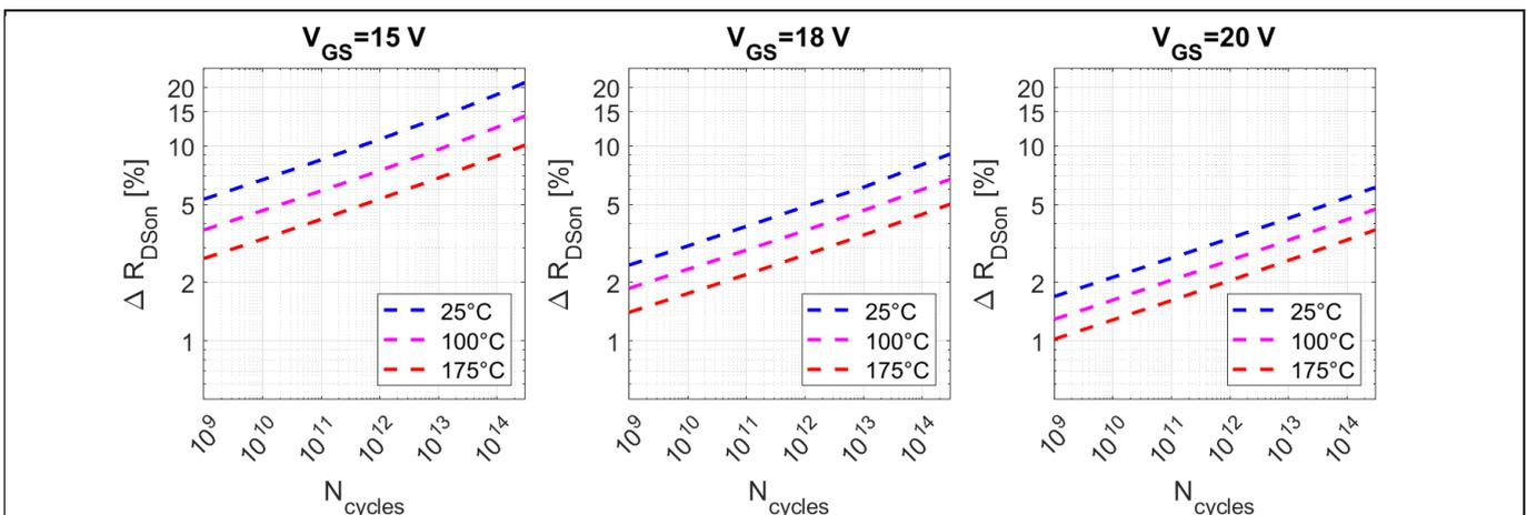
**Figure 7** Left: Relative  $R_{DS(on)}$  change at  $V_{GS(on)} = 15$  V,  $T_{j,op} = 25^{\circ}\text{C}$ ,  $100^{\circ}\text{C}$ , and  $175^{\circ}\text{C}$
