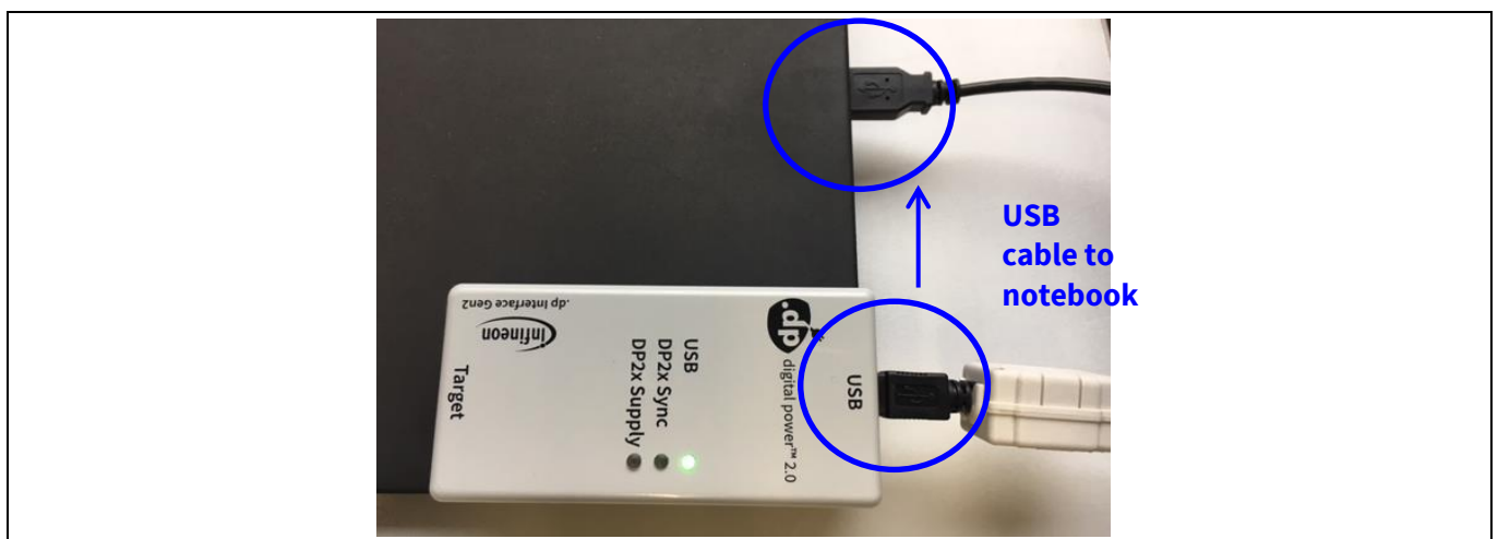
Figure 1 Connection between .dp Interface Gen2 and notebook
