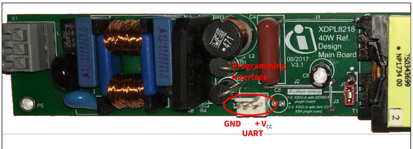
Figure 3 Connection between the .dp Interface Gen2 and the XDPL8210 reference board
