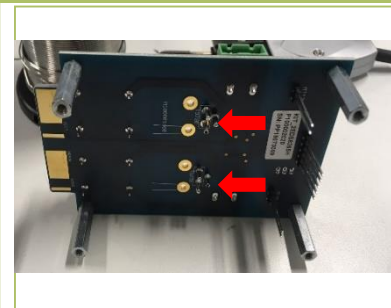
Step 8 Select the BS_EN jumper
