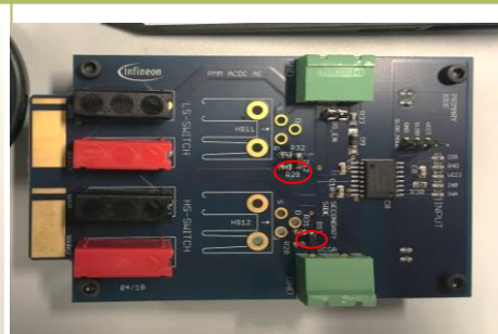
Step 7 Select the SLDO_MODE jumper
