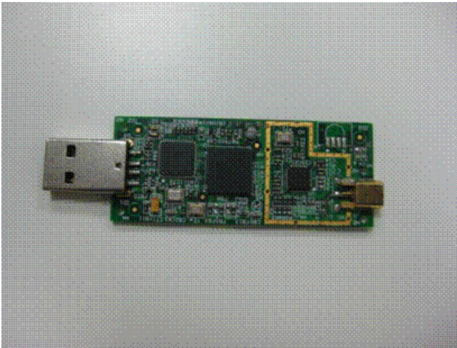
Sample CY_FX2LP_LGS_DMB-TH_TV Dongle Bottom View
