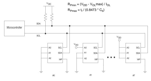
Figure 2. System Configuration using Serial (I<sup>2</sup>C) nvSRAM
