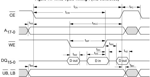
Figure 11. Write Cycle Timing 1 (WE Controlled) [10]
