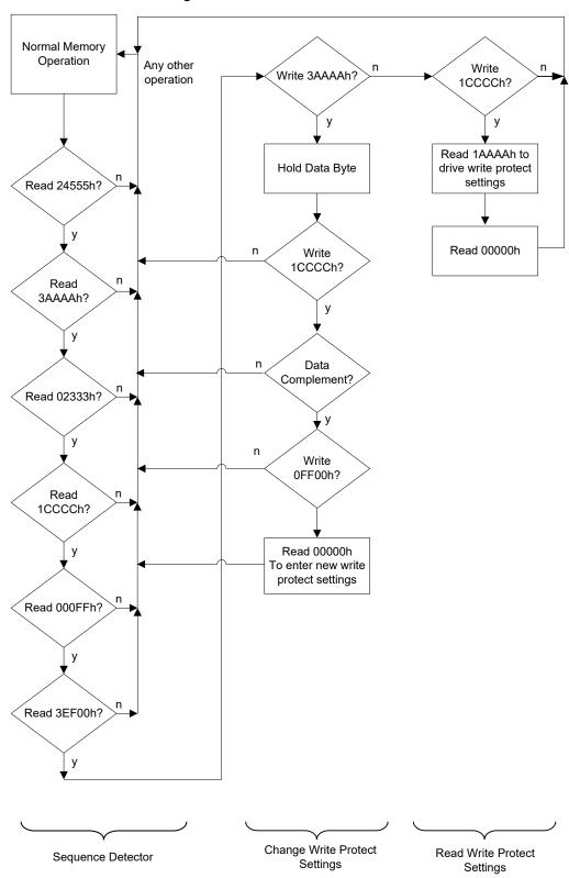
Figure 2. Write-Protect State Machine
