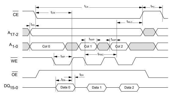
Figure 14. Page Mode Write Cycle Timing
