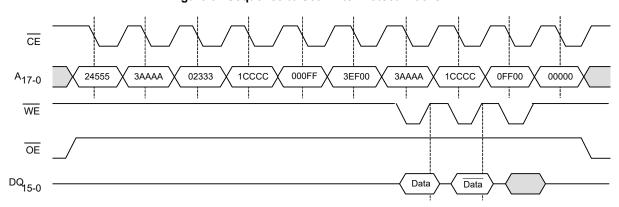
Figure 4. Sequence to Read Write-Protect Settings  $^{[1]}$
