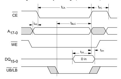
Figure 13. Write Cycle Timing 3 (CE LOW) [10]
