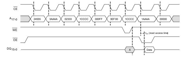
Note 1. This sequence requires  $t_{AS} \ge 10$  ns and address must be stable while  $\overline{CE}$  is LOW.
