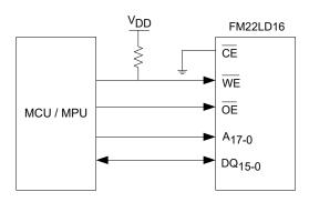
**Note** If  $\overline{CE}$  is tied to ground, the user gives up the ability to perform the software write-protect sequence.
