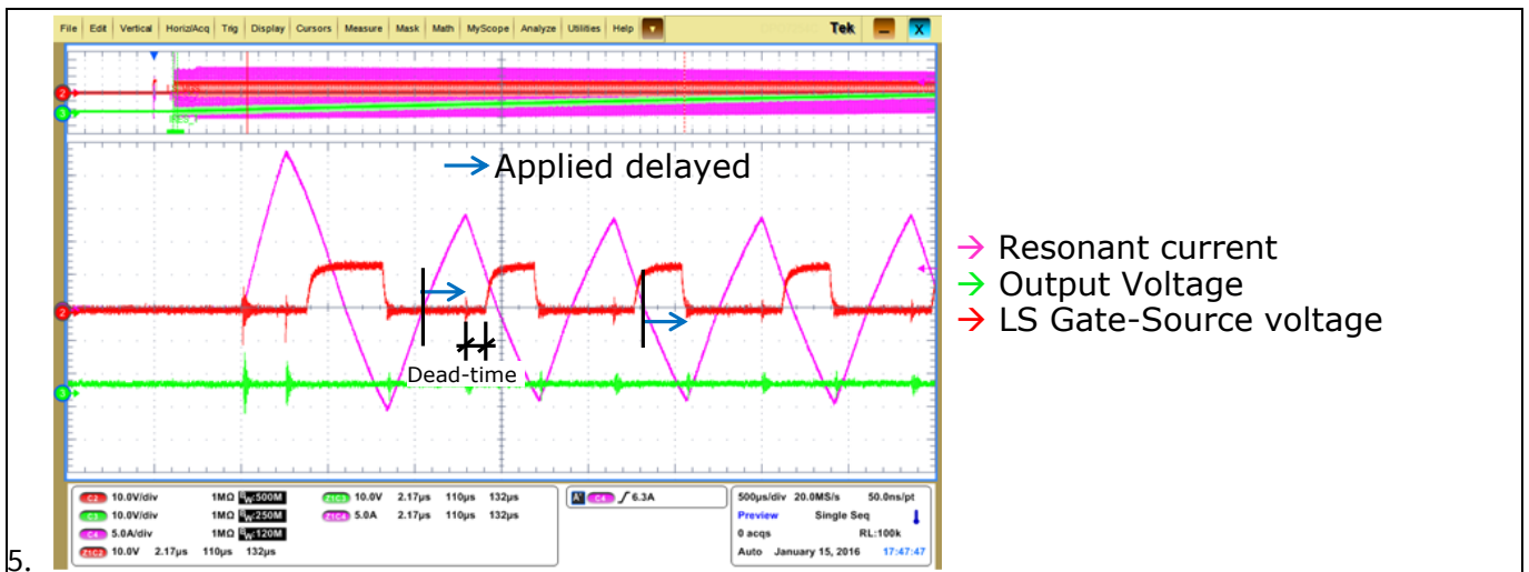
5. 6. Figure 27 LS-HS driving signal change is applied with a delay after the resonant current crosses zero to garrante current polarity change and avoid hard-conmuation.
