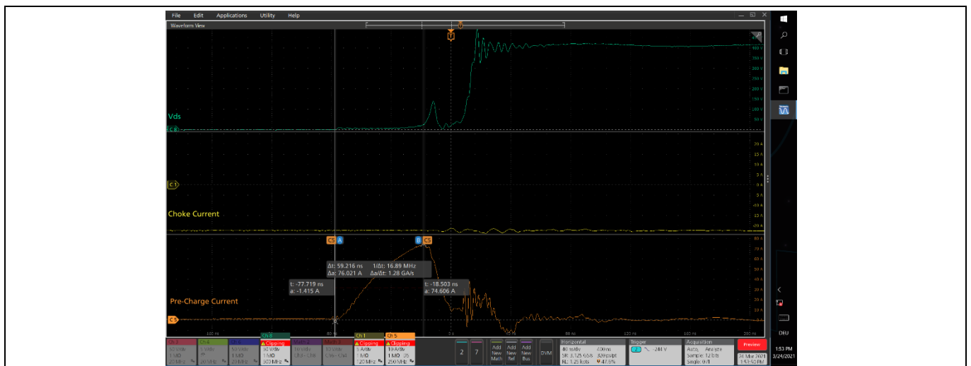
Figure 25 Pre-charge current and drain-source voltage of the CoolMOS™ CFD7 operating as a diode during totem pole operation and 23 A inductor current
