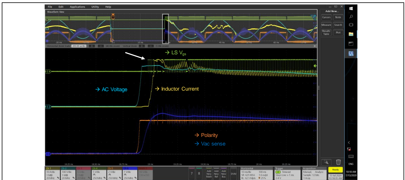
Figure 19 Low-side in the boost half-bridge is switched on first after the PWM is stopped
