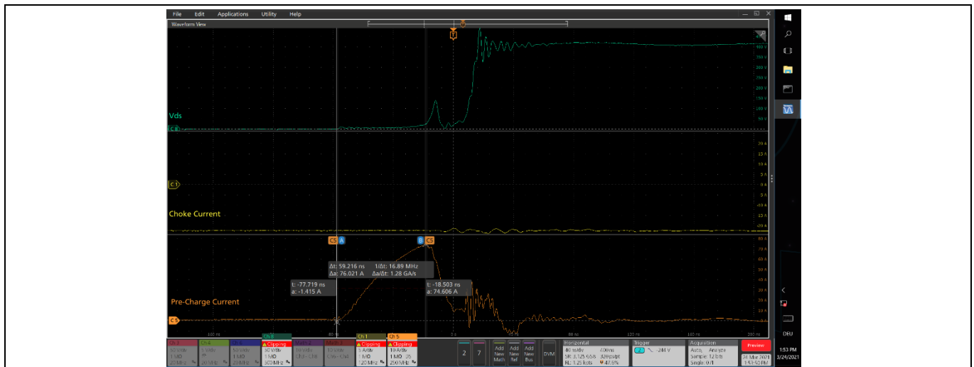
Figure 25 Pre-charge current and drain-source voltage of the CoolMOS™ CFD7 operating as a diode during totem pole operation and 23 A inductor current
