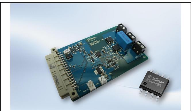
Figure 1 Top view of the EVAL-2EDL05I06PF
