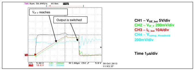
Figure 5 Over-current detection signals during simulated short circuit (current measured by Rogowski coil)
