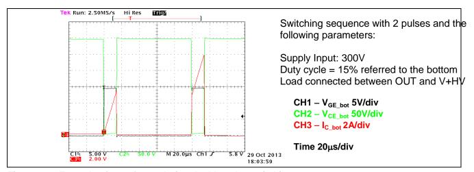
Figure 9 Example of waveforms during double pulse switching sequence
