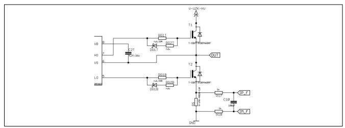
Figure 3 Shunt connection in the power circuit
