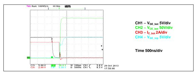
Figure 12 Turning off bottom IGBT and turning on top IGBT with delay of 500ns, load connected between OUT and GND\_HV, time scale 500ns/div (current measured by Rogowski coil)
