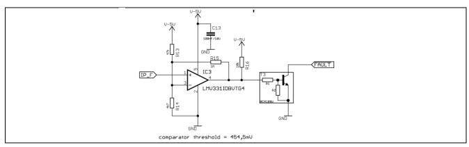
Figure 4 Overcurrent comparator circuit
