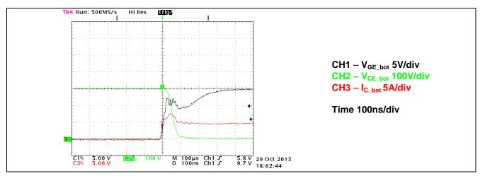
Figure 11 Turning on bottom IGBT, time scale 100ns/div (current measured by Rogowski coil)
