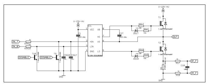
Figure 17 Infineon driver 2EDL05I06PF with shunt measurement
