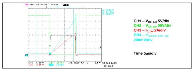
Figure 7 Current amplifier output and corresponding collector current (current measured by Rogowski coil)
