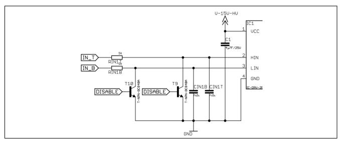
Figure 13 2EDL05I06PF gate driver input
