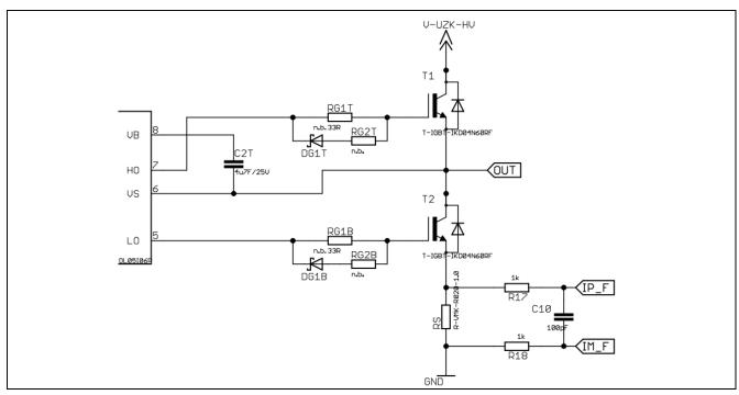
Figure 8 2EDL05I06PF gate driver output
