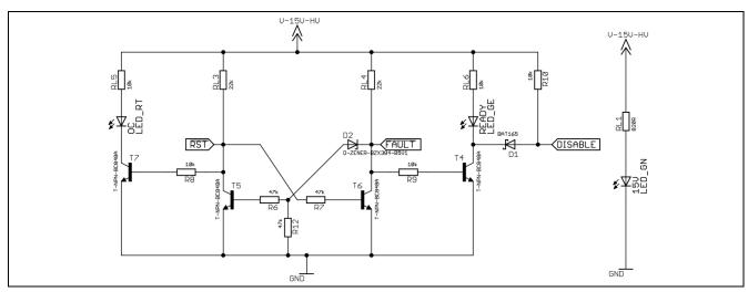
Figure 20 LEDs, FAULT and over current logic
