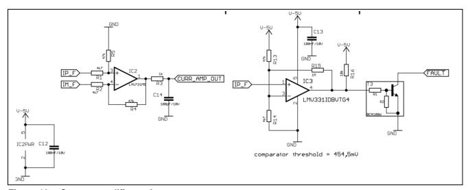
Figure 19 Current amplifier and overcurrent comparator
