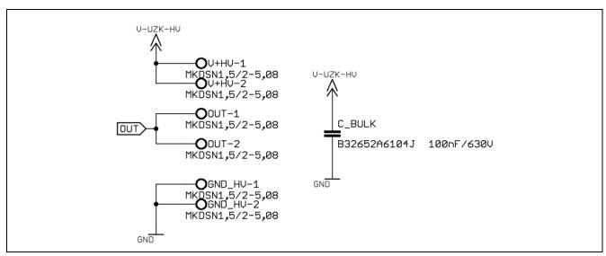
Figure 14 HV supply input and DC-Link
