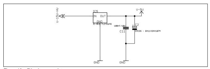
Figure 18 5V voltage regulator
