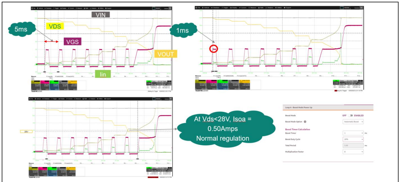
Figure 40 Automatic boost mode operation
