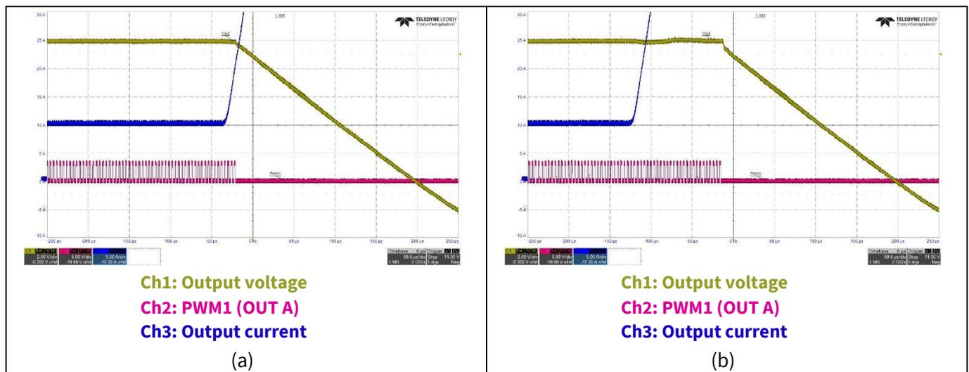
**Figure 37 Responses to SCP and OCP (at 48 V input, 12 V output)- a) shutdown by SCP, which responded in one switching cycle, b) shutdown by MFR\_IOUT\_OC\_FAST, which responded after 10 switching cycles**
