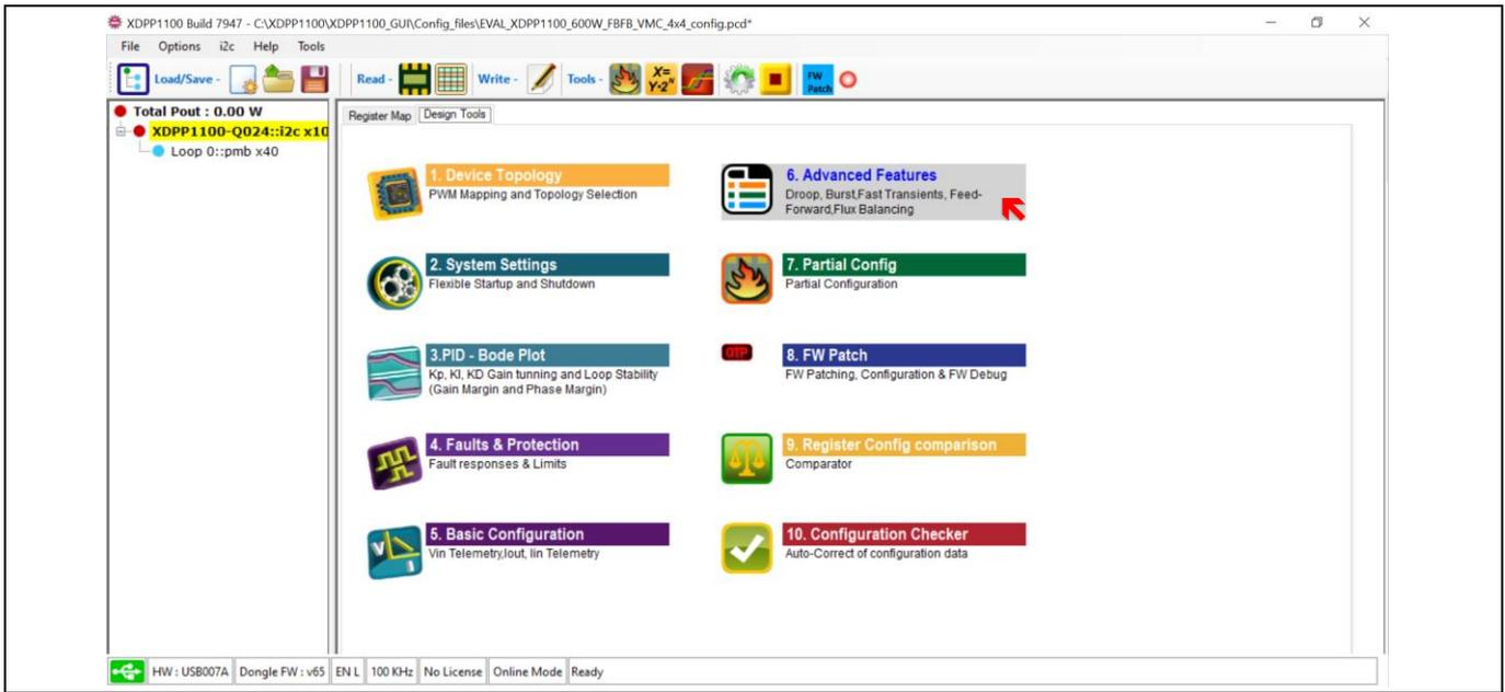
**Figure 49** Advanced features (droop, burst, fast transients, feed-forward, flux balancing)
