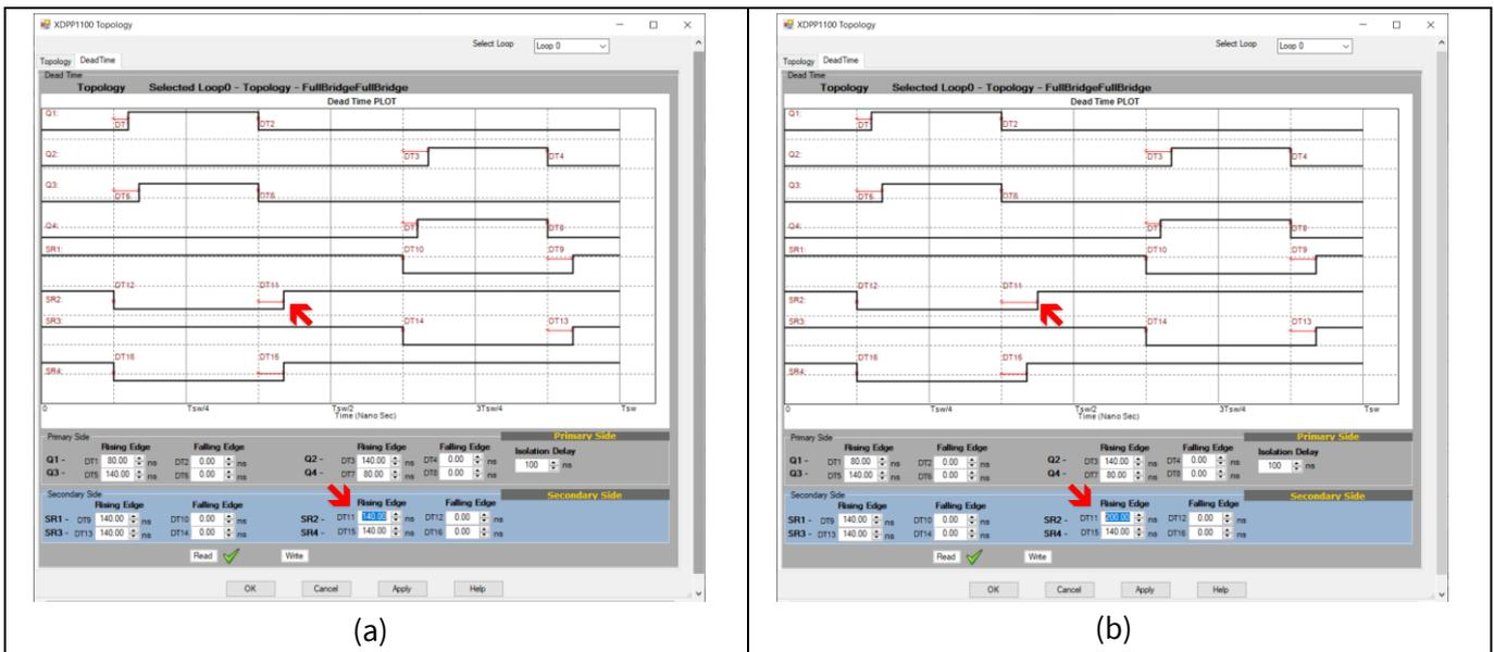
**Figure 18** PWM dead time configuration - a) DT11 = 140 ns, b) DT11 = 200 ns
