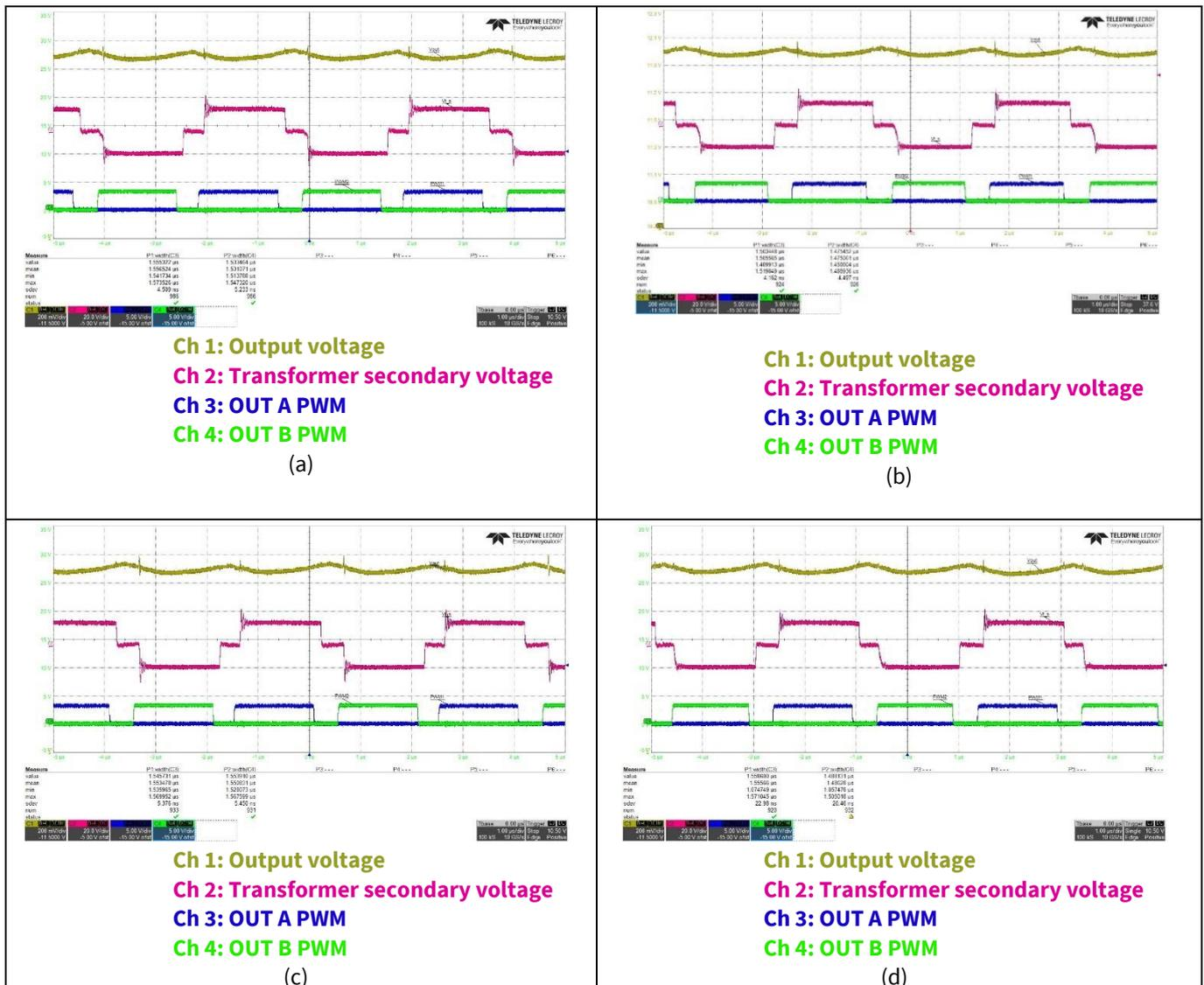
**Figure 52** Flux balancing steady-state result - a) ramp0\_dutyc\_lock = unchecked (flux balancing disabled), b) ramp0\_dutyc\_lock = checked and I<sub>OUT</sub> = 10 A (flux balancing is disabled due to DCM), c) ramp0\_dutyc\_lock = checked and fbal\_time\_only = enable (flux balancing is disabled due to DCM), d) ramp0\_dutyc\_lock = checked and fbal\_time\_only = disable (flux balancing enabled with volt × seconds technique)
