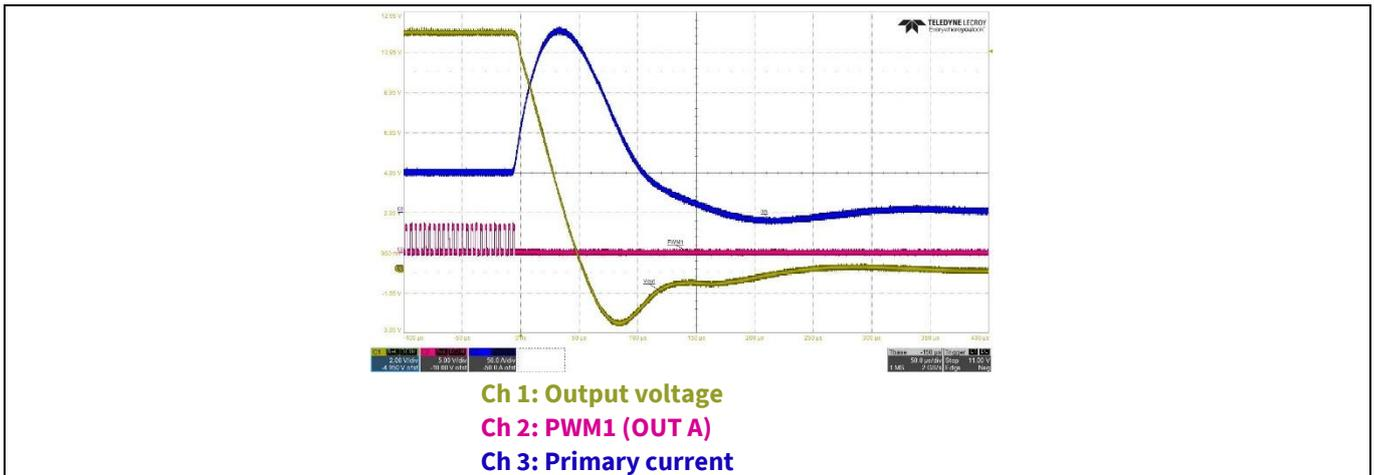
**Figure 40** Short-circuit protection
