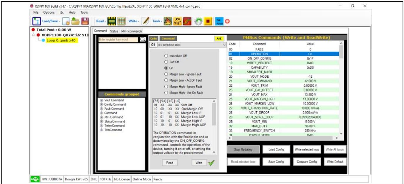
**Figure 13 PMBus OPERATION command**
