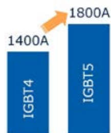
Figure 1: Extending the power range. Using the new PrimePACK 3+ package in conjunction with IGBT5 and emitter controlled diode 5
