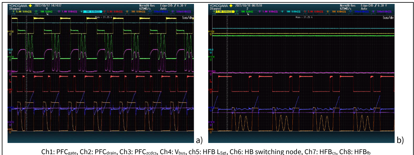
Figure 17 Continuous operation mode with HFB in ZV-RVS mode: a) PFC switching at third valley at 115 V input and 28 V 2 A output, and b) PFC disabled at 230 V, 15 V 1 A output
